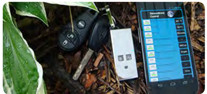
Sensordrone, which easily fits on a keychain, is a multisensor device developed by Sensorcon that collects and then transmits environmental data for analysis and display on a smartphone or tablet via Bluetooth. Several apps have already been created that turn the Sensordrone into a carbon monoxide monitor, weather monitor, and propane and other gas detectors — all in one device.
