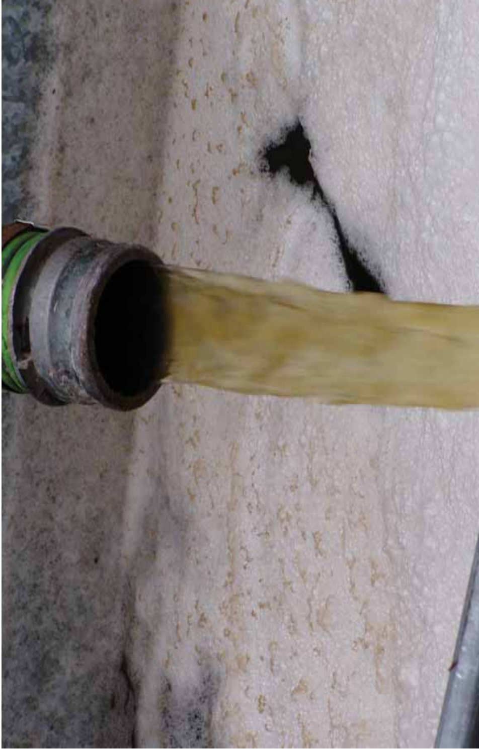
Clarified Filtrate discharging directly from Nutrient trap Process
