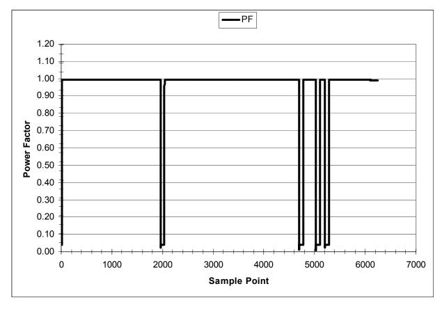
Figure 10-12 PEV 11B Power Factor over Charge Cycle
