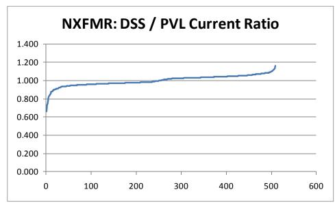
Figure 6-9 Ratio of OpenDSS to PVL Network Transformer Currents
