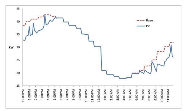
Figure 9-8 Transformer Loading with Photovoltaic Generation
