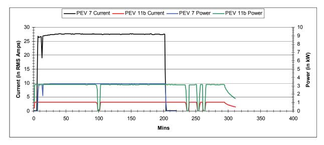
Figure 10-7 240V Charge Cycle
