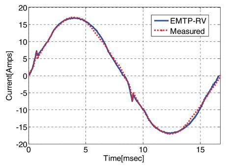
Figure 10-22 Comparison of Measured and Simulated Input Current Waveform
