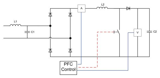
Figure 10-14 Circuit Topology of PFC Boost Converter
