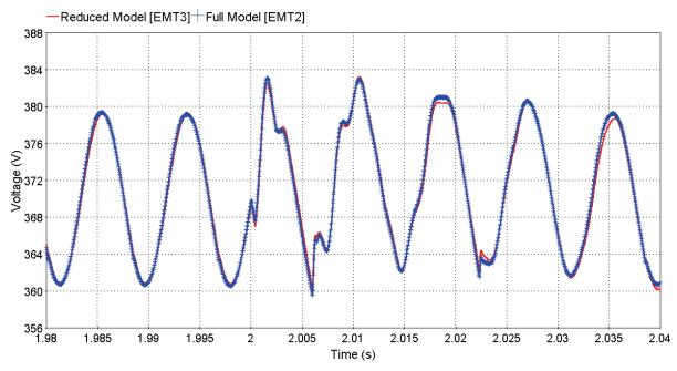
Figure 10-21 Comparison of Full Order and Reduced Order Boost Converter Model
