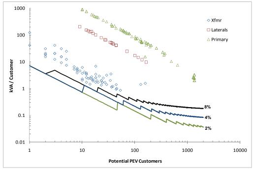
Figure 5-13 Feeder Asset Thermal Overload Risk Evaluation
