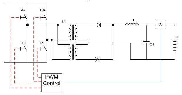
Figure 10-17 Circuit Topology of Full Bridge Forward Converter
