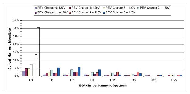
Figure 10-4 Harmonic Spectrum of 120V Chargers
