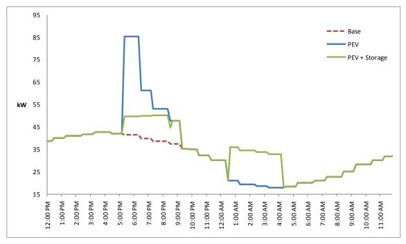
Figure 9-7 Transformer Loading when PEV and Storage are Connected
