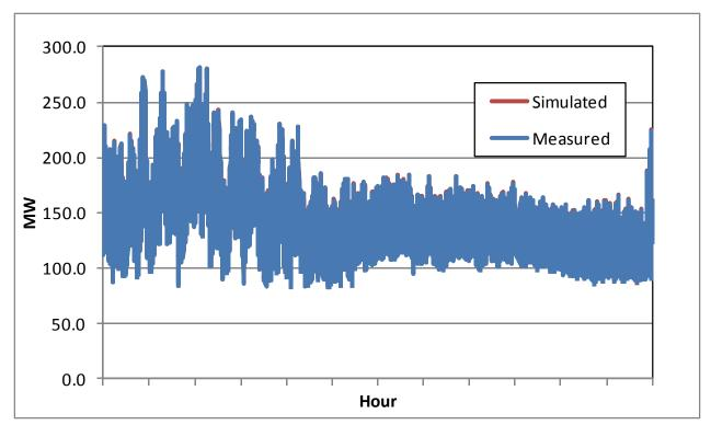
Figure 5-8 Model Validation of Feeder Current
