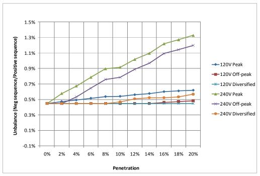
Figure 5-17 System Deterministic Case Voltage Unbalance Factors
