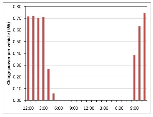
Figure 4-11 Average PEV Loading for Customer Behavior with simple charge control
