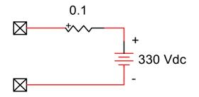
Figure 10-19 Time Domain Battery Model
