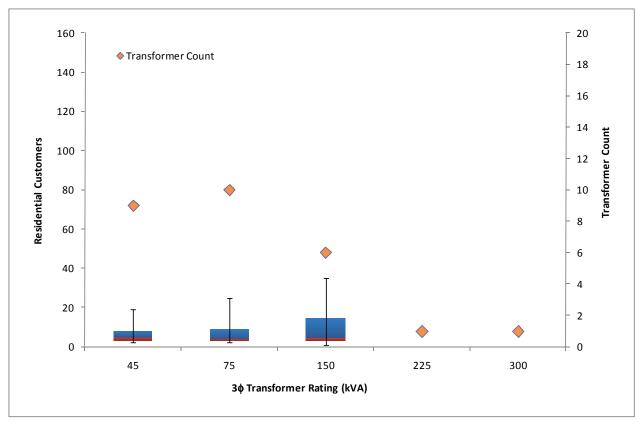
Figure 5-7 Three-Phase Transformer and Residential Customer Feeder Allocation
