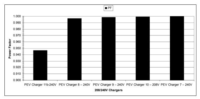
Figure 10-11 208/240V Charger System Power Factor
