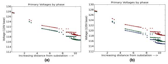
Figure 5-16 Feeder Peak-Hour Voltage Profiles (a) Base Case (b) 8% Market Worst-case
