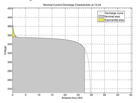
Figure 10-20 Discharge Characteristics of a 330 V, 10 kWh, Li ion Battery
