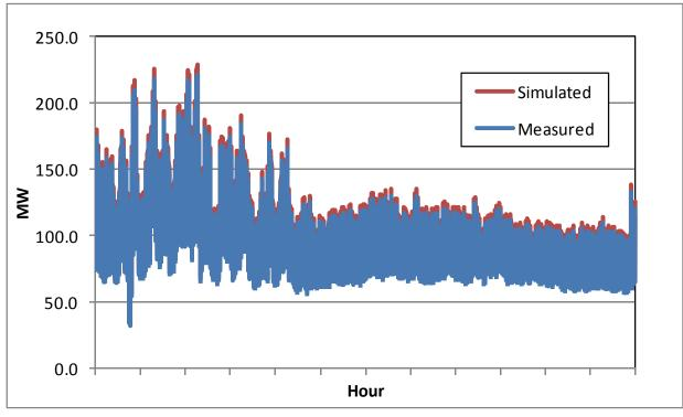
Figure 5-9 Model Validation of Total Substation Total Load
