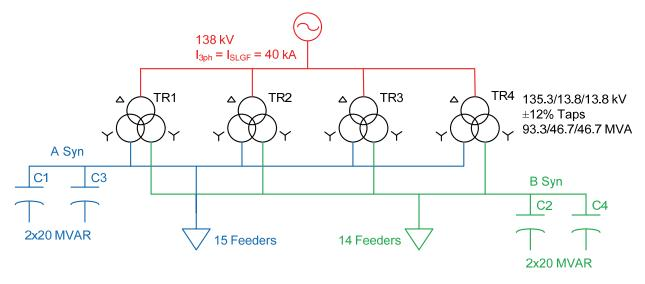
Figure 6-4 Simplified One-line Diagram of the Hellgate Substation
