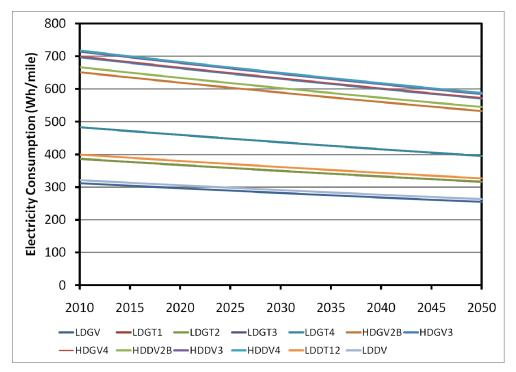
Figure 3-3 Electricity Consumption for PEVs
