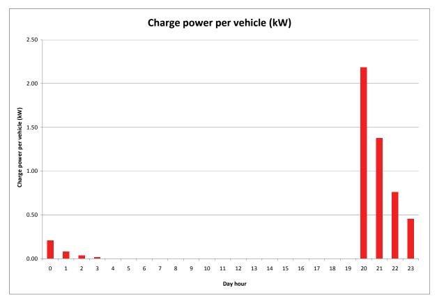
Figure 4-12 Average PEV Loading for Incorrectly controlled electric vehicle charging load
