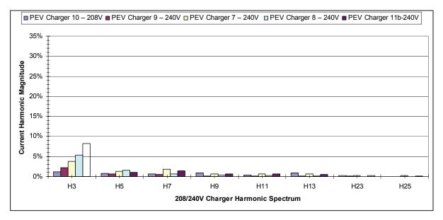
Figure 10-5 Harmonic Spectrum of 208/240V Charger Systems
