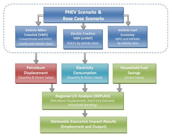
Figure 7-1 Schematic Overview of Study Methodology
