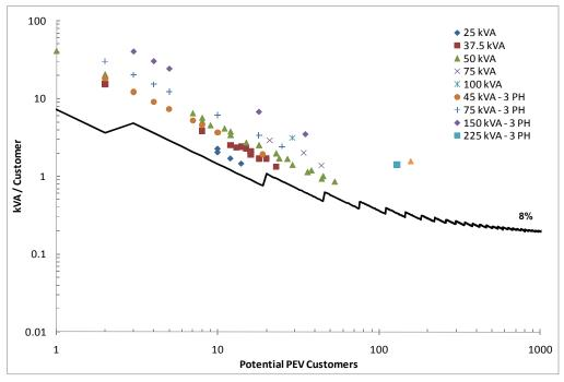
Figure 5-14 Service Transformer Overload Risk Evaluation
