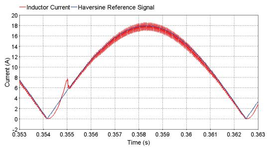
Figure 10-16 Comparison of Inductor Current with Reference Signal
