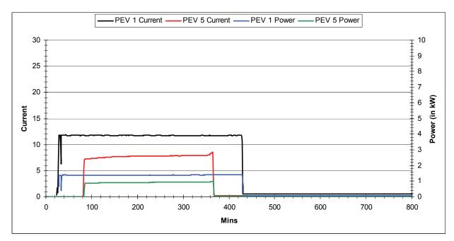
Figure 10-6 120V Charge Cycle
