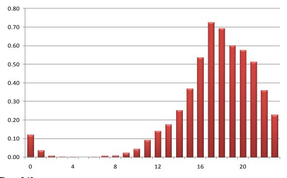
Figure 5-12 Average Hourly (Charge Power per Vehicle) Projected Plug-In Electric Vehicle Demand
