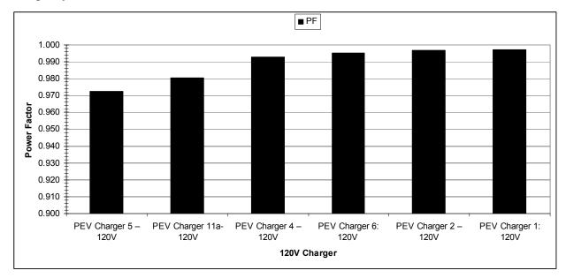
Figure 10-10 120V Charger System Power Factor
