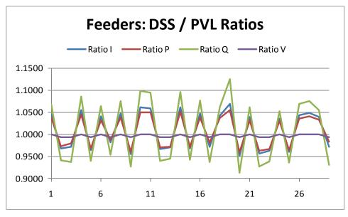
Figure 6-10 Ratio of OpenDSS to PVL Primary Feeder Voltage and Flow Quantities
