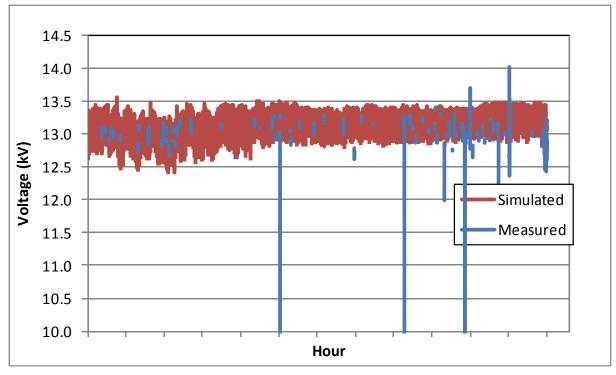
Figure 5-11 Model Validation of Tie Point Voltage
