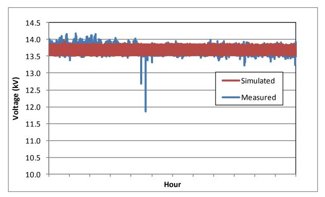
Figure 5-10 Model Validation of Harrison Substation Voltage
