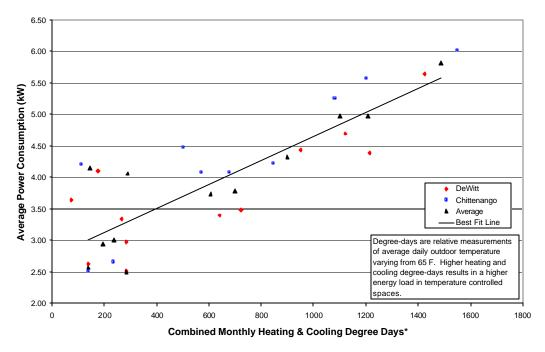
Figure 18. Average Power Consumption per Number of Monthly Degree Days
