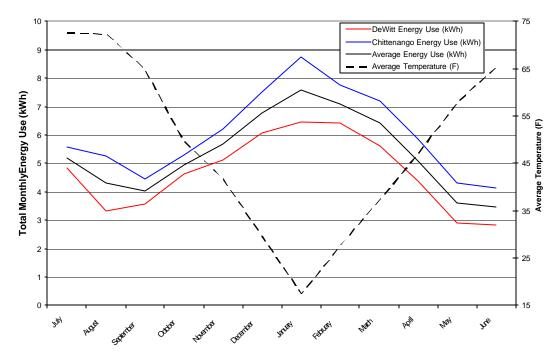
Figure 14: Monthly Average Energy Usage and Temperatures
