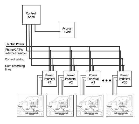
Figure 4: Shorepower TSE system diagram
