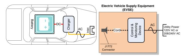
There are three distinct levels of EV charging in widespread use—Level 1 (120V), Level 2 (208 / 240 V), and DC fast charging (208-480 V). Table A-1 lists their specifications, and the subsequent sections provide further description. Using common standards for charging has greatly aided the adoption of EVs and the development of charging infrastructure. Figures A-2 through A-4 provide charging method examples.
