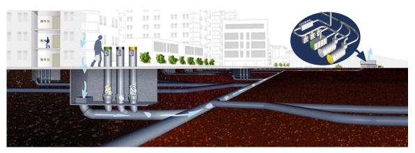
Figure 1-9. Three-Way Diverter Valve (Source: Kogler, 2007)
