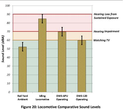
is approximately 45-55 decibels (dB). Once the locomotive's diesel engine was started, the readings were 65-90 dB. With the idle reduction technology, the noise readings were 45-62 dB for the DWS-120 and 45-72 dB for the DWS-APU.
