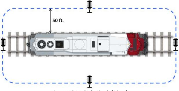
Figure 5: Noise Reading locations (50ft Shown)
