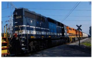
Figure 14: RSR Locomotive #3106 with a DWS-APU
