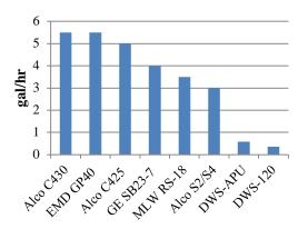
Figure 3: Average Fuel Consumption of Locomotives and the DWS at Idle
