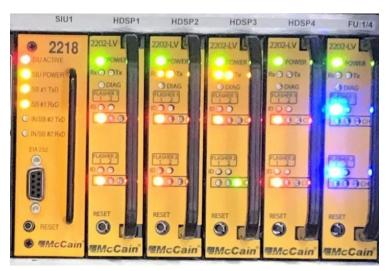
Figure 2. High-Density Switch Packs and Serial Interface Unit
