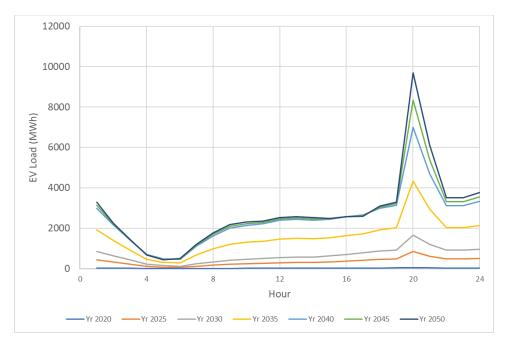
Figure 12. Managed EV Charging Profile for the LDI Scenario
