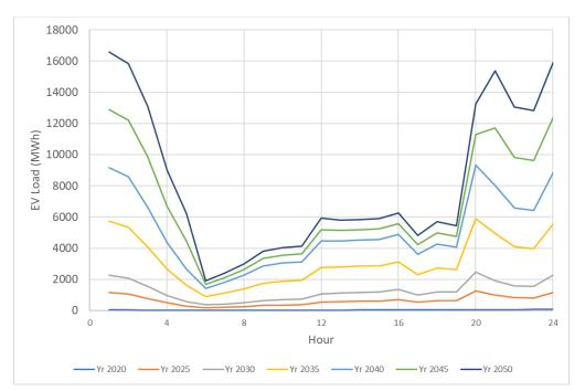
Figure 8. Managed EV Charging Profile for the HDI Scenario
