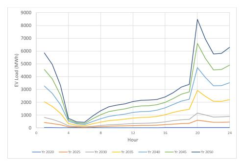
Figure 4. Managed EV Charging Profile for the Reference Scenario
