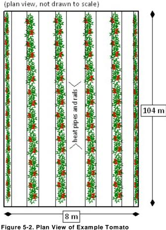
Figure 5-2. Plan View of Example Tomato Greenhouse
