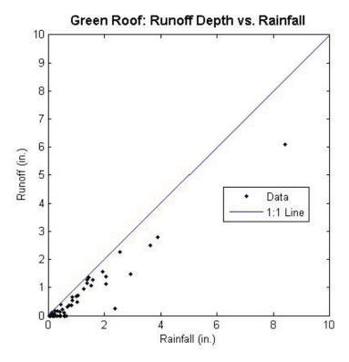
Figure 46: Scatter plot of green roof runoff versus precipitation for rainfall events from 10/1/06 to 10/1/07.
