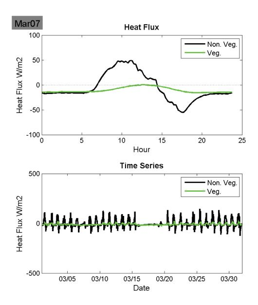
**Figure 32:** March 2007 Average diurnal heat flux through a green and non-green roof (top) and monthly daily heat flux.
