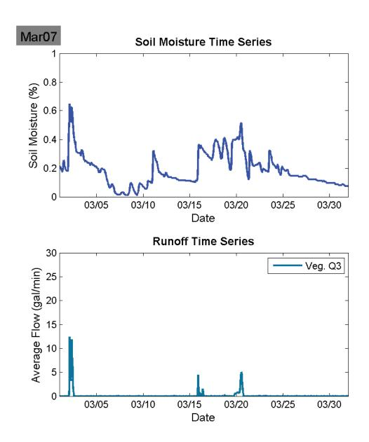
Figure 54: March 2007 Soil moisture (%) and Veg. Q3 runoff (gal/min).
