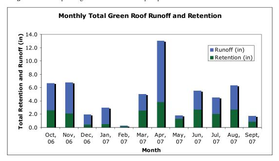
**Figure 47:** Monthly runoff and retention of stormwater by the Gratz green roof in New York City. Total bar (Runoff + Retention) height is equal to the total precipitation for events measured during each month.
