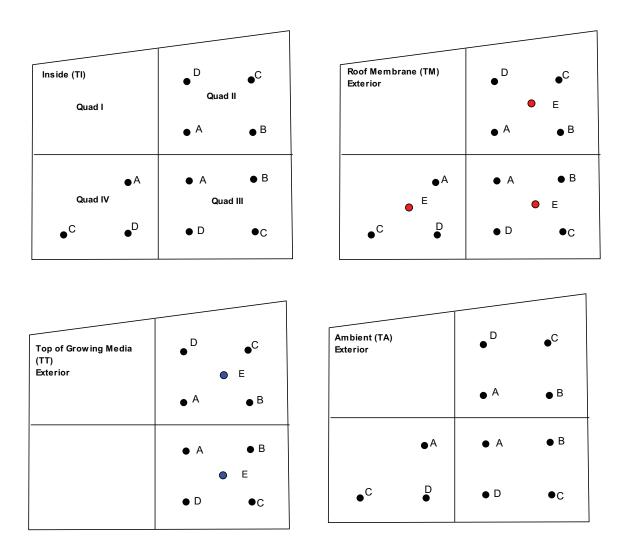
**Figure 3: Sensor placement.** Layout of thermocouples ( ●): exterior, interior and vertical locations in the quadrants (A, B, C, & D). E is the location for heat flow sensors ( ● - on the roof membrane) and in the vegetated quadrants, the water content reflectometers ( ● - in the growing media).
