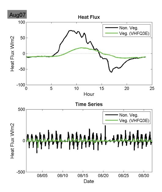
**Figure 42:** August 2007 Average diurnal heat flux through a green and non-green roof (top) and monthly daily heat flux.
