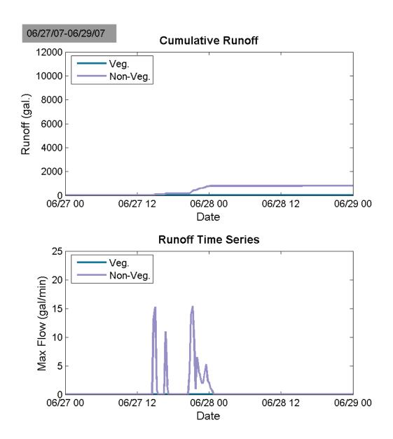
Figure 63: Runoff from control and vegetated roof sections for a typical summer rain of under  $\frac{1}{2}$  inch ( $\sim$ 10 mm).
