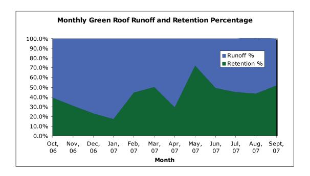
**Figure 48:** Stormwater runoff and retention as a percentage of the total precipitation of measured events for each month.
