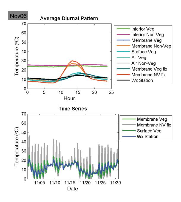
Figure 23: November 2006 Average diurnal temperatures (top) and monthly average temperatures.
