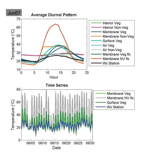
Figure 37: June 2007 Average diurnal temperatures (top) and monthly average temperatures.
