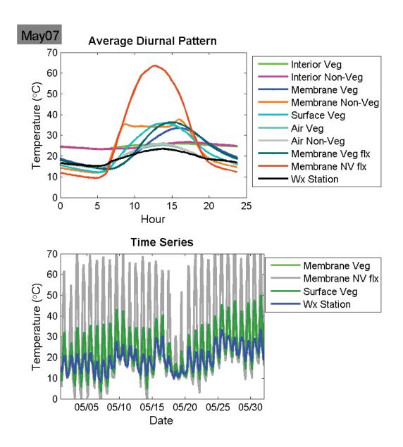
Figure 35: May 2007 Average diurnal temperatures (top) and monthly average temperatures.
