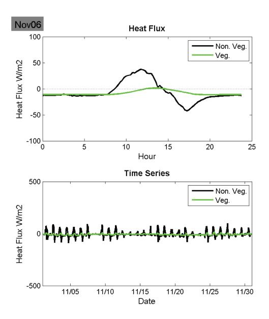
**Figure 24:** November 2006 Average diurnal heat flux through a green and non-green roof (top) and monthly daily heat flux.
