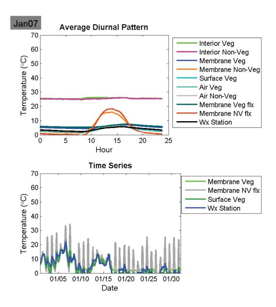
Figure 27: January 2007 Average diurnal temperatures (top) and monthly average temperatures.
