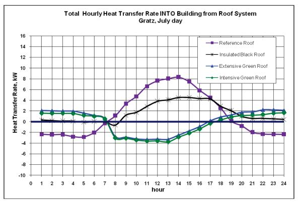
Figure 13: Total Hourly Heat Transfer Rate Into Building, Gratz (July)
