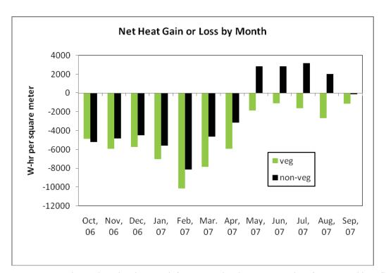
**Figure 20:** Net heat gain or loss by month for vegetated and non-vegetated roof. Vegetated heat flux sensor averages were used for Oct 2006-May 2007. Due to sensor failure, only VHFQ3E (veg. quad III) data were used for June-September 2007.
