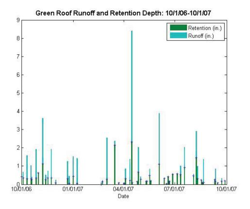
**Figure 45:** Runoff and retention of measured precipitation events by the Gratz green roof in New York City. The total bar height (Runoff + Retention) is equal to the measured precipitation.
