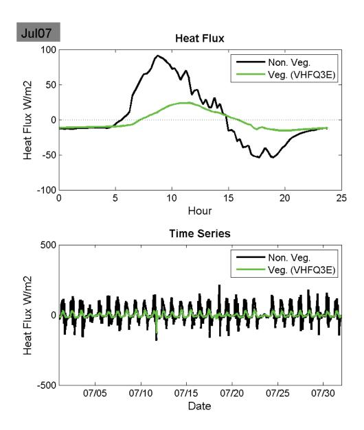
**Figure 40:** July 2007 Average diurnal heat flux through a green and non-green roof (top) and monthly daily heat flux.
