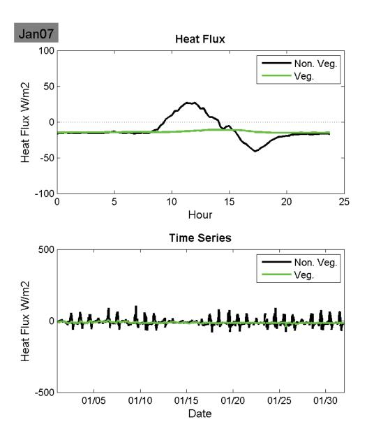
**Figure 28:** January 2007 Average diurnal heat flux through a green and non-green roof (top) and monthly daily heat flux.
