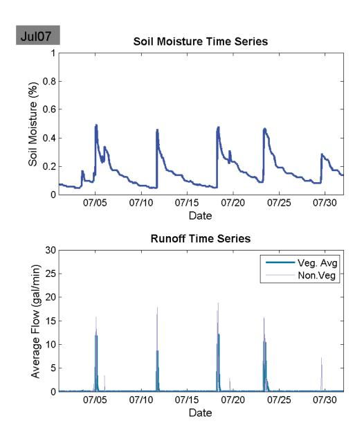
Figure 58: July 2007 Soil moisture (%) and Veg. Avg. runoff (gal/min).
