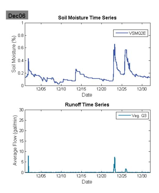
**Figure 51:** December 2006 Soil moisture (%) and Veg. Q3 runoff (gal/min). The quadrant III soil moisture (VSMQ3E) probe malfunctioned in this month, so in place of an average, only the quadrant II soil moisture (VSMQ2E) is shown.
