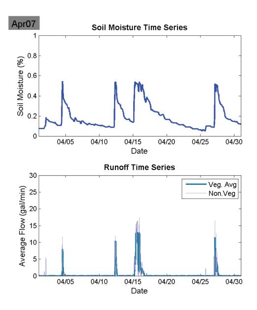
Figure 55: April 2007 Soil moisture (%) and Veg. Avg. runoff (gal/min).
