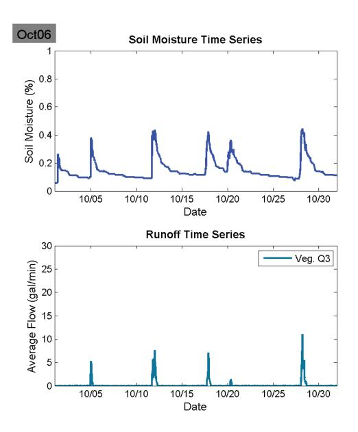
Figure 49: October 2006 Soil moisture (%) and Veg. Q3 runoff (gal/min).
