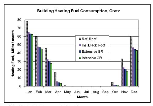
Figure 19: Building Heating Fuel Consumption, Monthly
