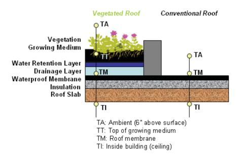
Figure 2: Vertical placement of thermocouples.
