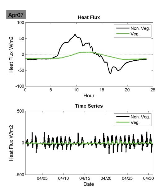
**Figure 34:** April 2007 Average diurnal heat flux through a green and non-green roof (top) and monthly daily heat flux.
