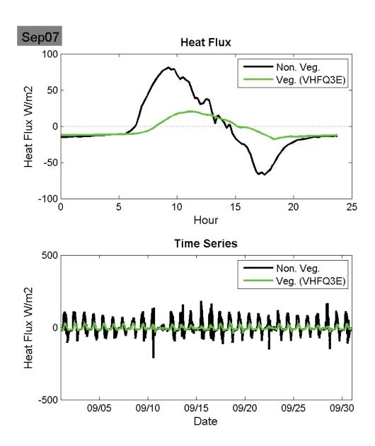
**Figure 44:** September 2007 Average diurnal heat flux through a green and non-green roof (top) and monthly daily heat flux.
