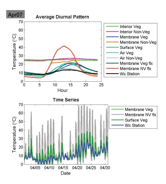
Figure 33: April 2007 Average diurnal temperatures (top) and monthly average temperatures.
