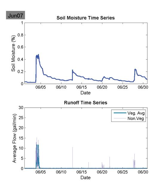
Figure 57: June 2007 Soil moisture (%) and Veg. Avg. runoff (gal/min).
