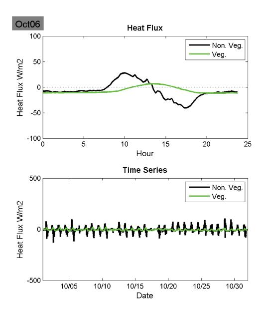
**Figure 22:** October 2006 Average diurnal heat flux through a green and non-green roof (top) and monthly daily heat flux.
