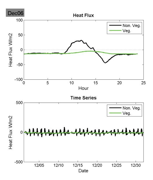
**Figure 26:** December 2006 Average diurnal heat flux through a green and non-green roof (top) and monthly daily heat flux.
