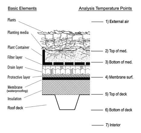
Figure 4: Green Roof Layer Diagram
