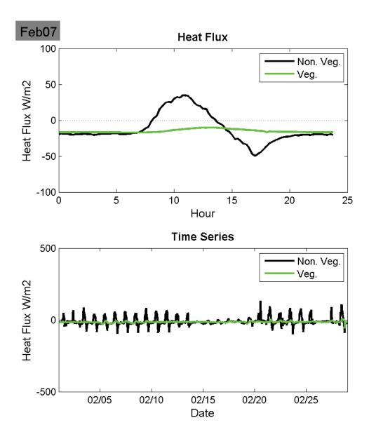
**Figure 30:** February 2007 Average diurnal heat flux through a green and non-green roof (top) and monthly daily heat flux.
