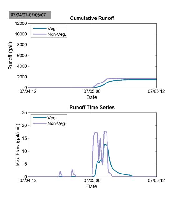
Figure 62: Runoff from vegetated and non-vegetated control roofs for a 1.4" summer rain.
