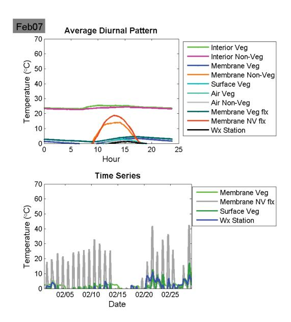
Figure 29: February 2007 Average diurnal temperatures (top) and monthly average temperatures.
