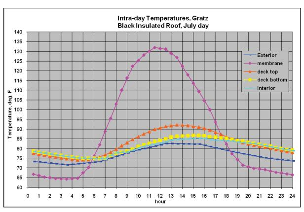
Figure 6: Intra-dayTemperatures, Gratz Black Insulated Roof
