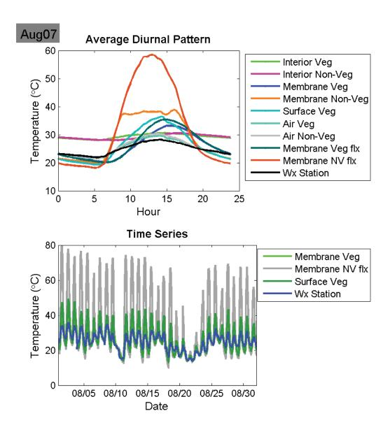
Figure 41: August 2007 Average diurnal temperatures (top) and monthly average temperatures.
