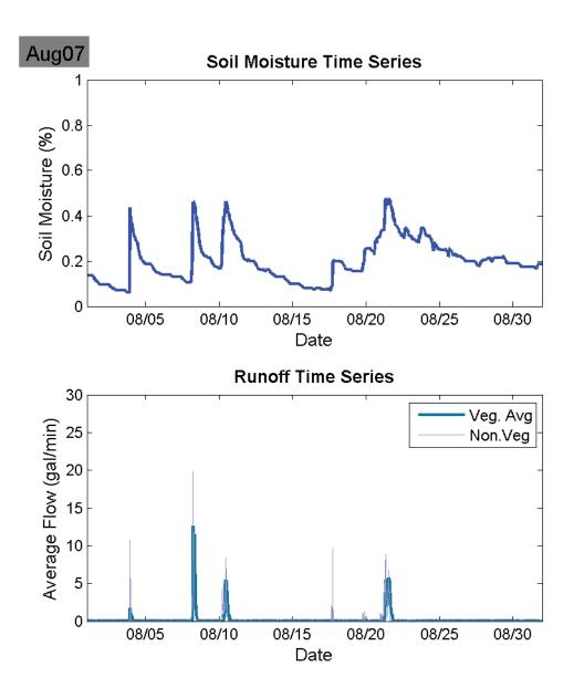
Figure 59: August 2007 Soil moisture (%) and Veg. Avg. runoff (gal/min).
