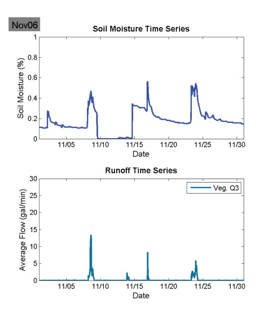
Figure 50: November 2006 Soil moisture (%) and Veg. Q3 runoff (gal/min).
