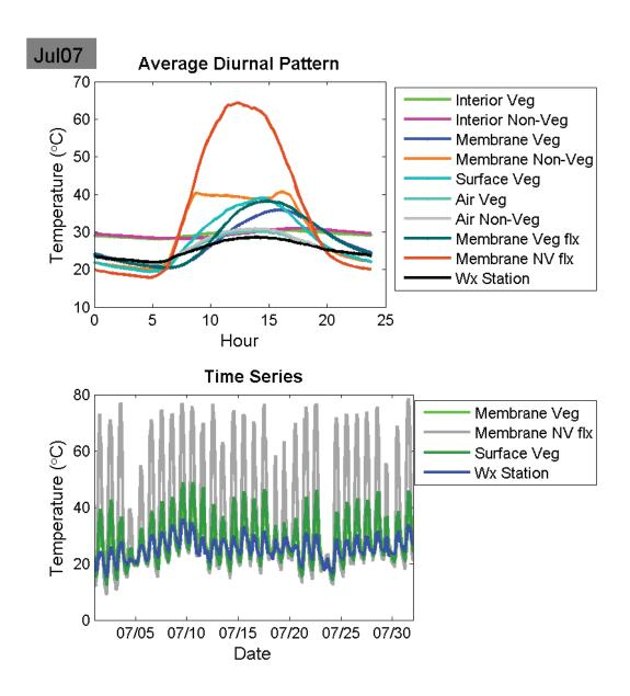
Figure 39: July 2007 Average diurnal temperatures (top) and monthly average temperatures.
