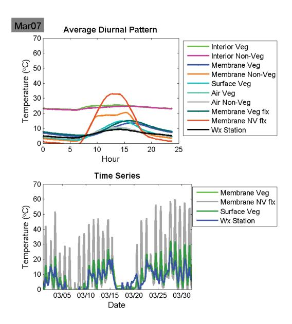
Figure 31: March 2007 Average diurnal temperatures (top) and monthly average temperatures.
