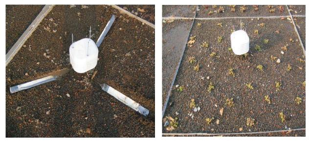
Installation of Heat Flow Sensor and Water Content Reflectometer
