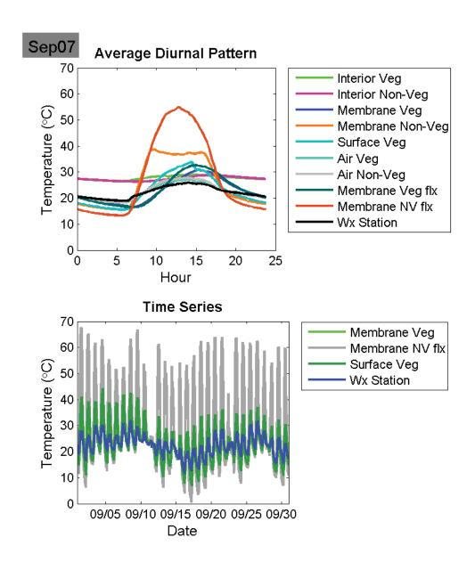
Figure 43: September 2007 Average diurnal temperatures (top) and monthly average temperatures.
