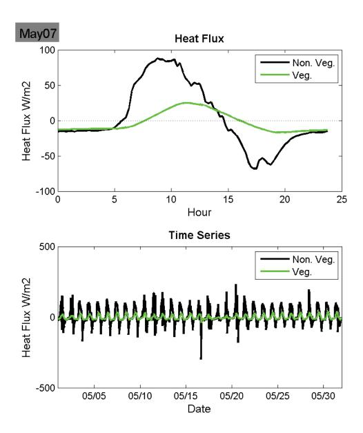
**Figure 36:** May 2007 Average diurnal heat flux through a green and non-green roof (top) and monthly daily heat flux.
