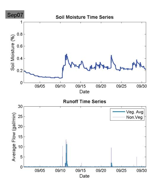
Figure 60: September 2007 Soil moisture (%) and Veg. Avg. runoff (gal/min).
