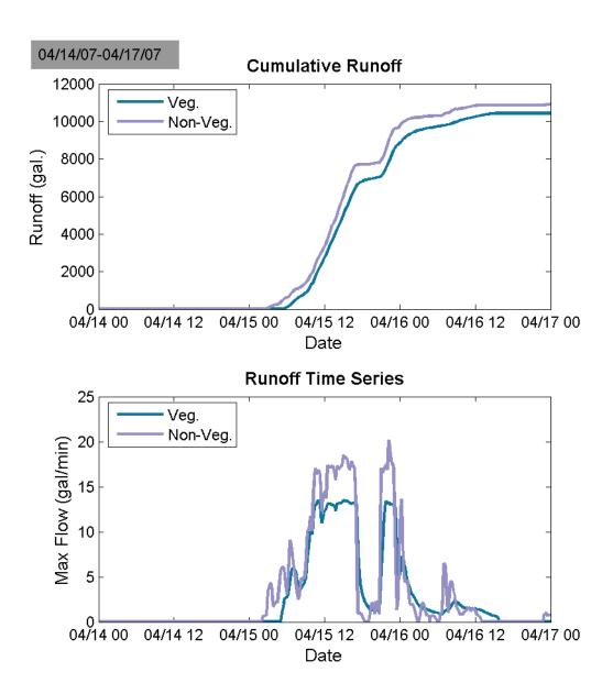
Figure 61: Runoff from Gratz vegetated and non-vegetated control roofs. Total precipitation in excess of 8".
