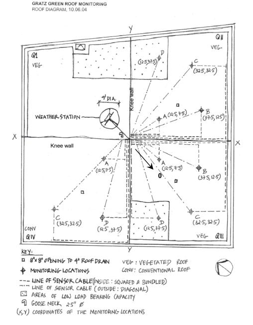
**Figure 1:** Roof plan and horizontal monitoring locations. The numbers are absolute values, in feet, from the origin '0'.
