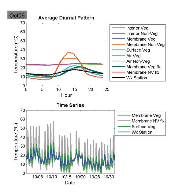
Figure 21: October 2006 Average diurnal temperatures (top) and monthly average temperatures.
