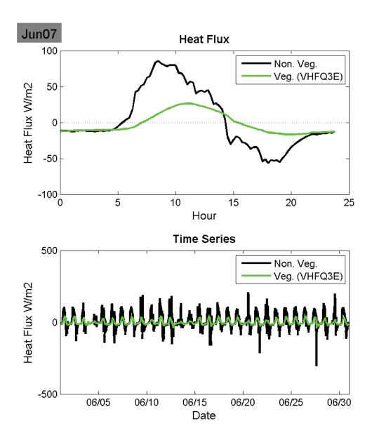
**Figure 38:** June 2007 Average diurnal heat flux through a green and non-green roof (top) and monthly daily heat flux.
