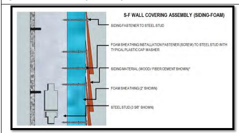
Option #2, Means (a) - Siding to Stud
