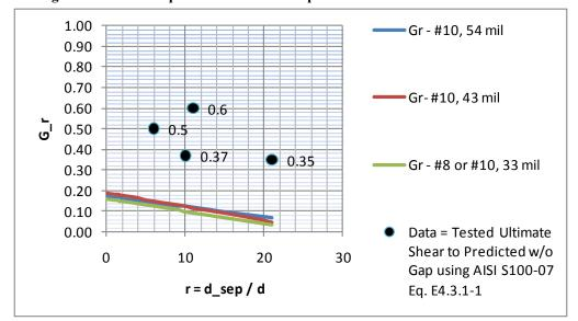
Figure 27. Plot of Gap Reduction Factor Equations vs. Test Data at Failure Load
