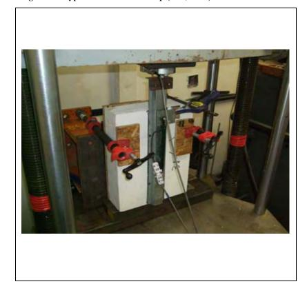
Figure 19. Typical Shear Test Set-up (PEI, 201a)
