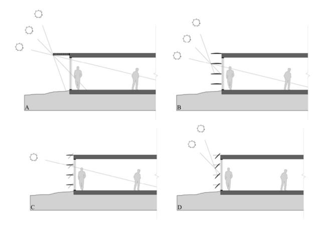
Figure 2g – Illustrations of different shading options – (A) Fixed overhang at 4 feet (B) Fixed louver at 2.5 feet (C) Winter operable louver at 1.75 feet (D) Summer operable louver at 1.75 feet
