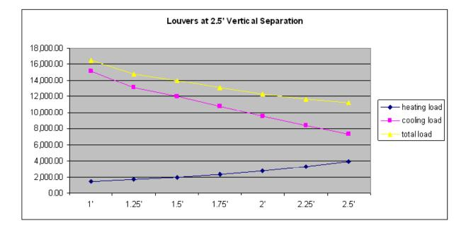
Figure 2d - Chart illustrating heating and cooling trends when altering louver projections.
