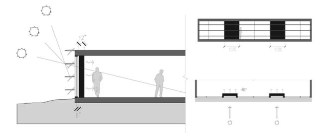
Figure 2h – Illustrations of optimum trombe application (correct louvers, cavity spacing, trombe width and a 30% trombe/70% glazing elevation and plan)
