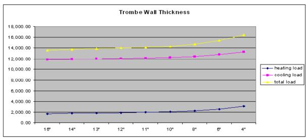
Figure 2b - Chart illustrating heating and cooling trends when altering trombe thickness.
