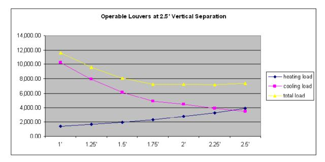
Figure 2e - Chart illustrating heating and cooling trends when altering operable louver projections.
