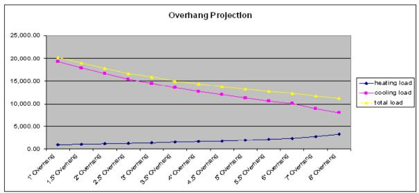
Figure 2c - Chart illustrating heating and cooling trends when altering overhang projections.
