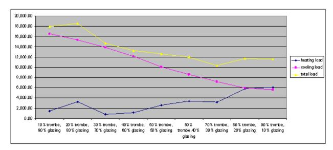
Figure 2 - Chart illustrating heating and cooling trends when altering trombe-to-glazing ratios.
