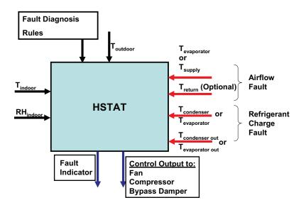
Figure 1-2 A Schematic Illustration of the HSTAT Concept Developed by SWA under a DOE SBIR Project.
