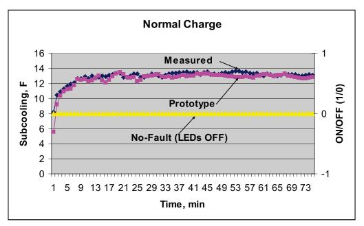
Figure 4-7 Subcooling Profile Along with ON/OFF Status for the Normal Charge Case.
