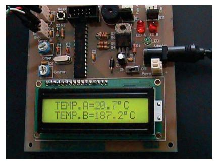
Figure 2-10 The Differential Temperature Prototype in Operation before Fault Detection Algorithm was Programmed.
