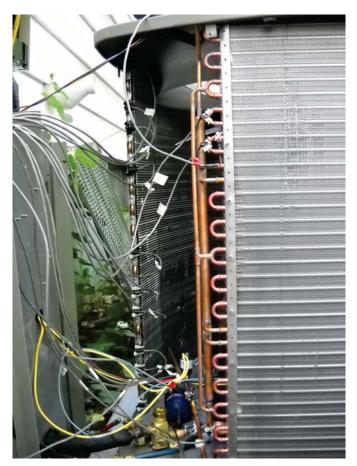
Figure 3-3 Condenser Coil (Outdoor Unit) with Temperature Sensors Placed.
