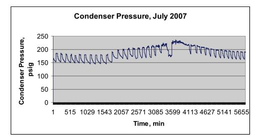
Figure 2-3 A Condenser Pressure Profile of an R-22 System.
