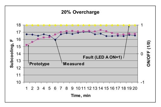
Figure 4-11 Subcooling Profile Along with ON/OFF Status for the 20% Overcharge Case.
