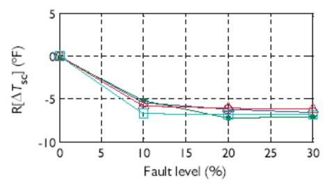
Figure 3-11 Refrigerant Subcooling Change as a Function of Undercharge (NIST data [15]).
