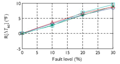
Figure 3-12 Refrigerant Subcooling Change as a Function Overcharge (NIST data [15]).
