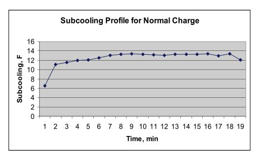
Figure 3-6 Refrigerant Subcooling as a Function of Time for Normal Charge.
