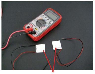
**Thermoelectric Modules** Figure 2-6 Thermoelectric Modules for Measuring Subcooling.
