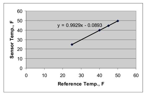
Figure 2-12 Agreement Between the Prototype's Temperature Sensor and the Reference Temperature.
