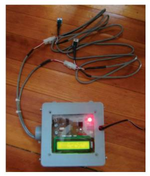
Figure 4-4 Field-Ready Refrigerant Charge Fault Detector Prototype Built by SWA.
