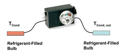
Figure 2-1 A Concept Using Differential Pressure for Detecting Subcooling.
