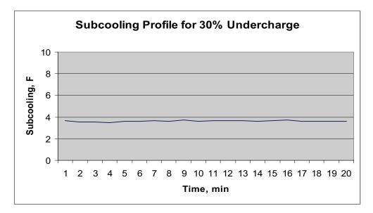
Figure 3-9 Refrigerant Subcooling as a Function of Time for 30% Undercharge.
