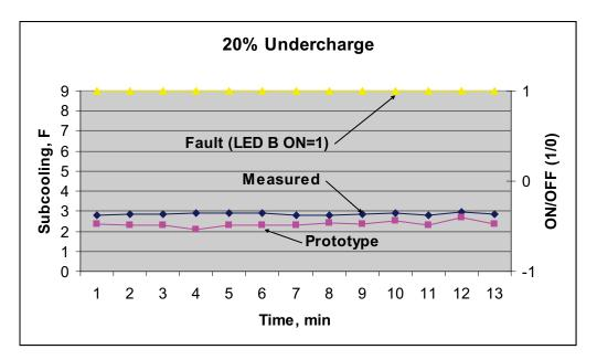
Figure 4-9 Subcooling Profile Along with ON/OFF Status for the 20% Undercharge Case.
