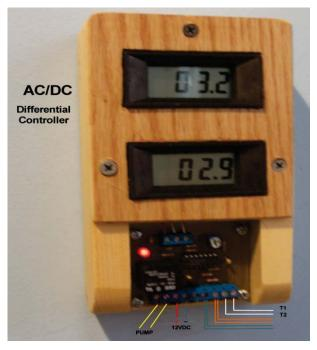
Figure 2-8 A Differential Controller Kit Evaluated by SWA for Sensing Subcooling.
