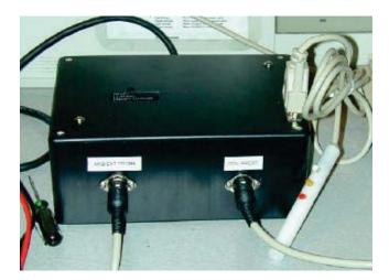
Figure 4-1 A Pre-Prototype Charge Detector Built by Oak Ridge National Laboratory.
