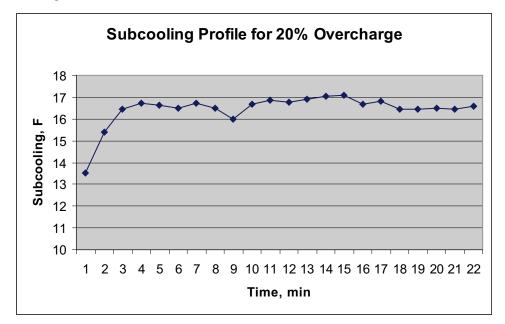
Figure 3-10 Refrigerant Subcooling as a Function of Time for 20% Overcharge.
