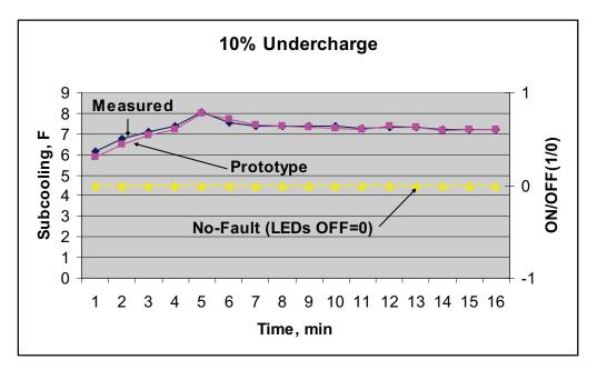
Figure 4-8 Subcooling Profile Along with ON/OFF Status for the 10% Undercharge Case.
