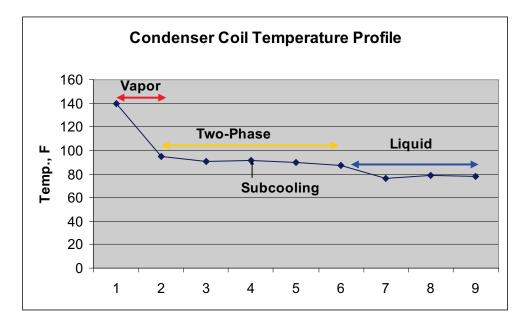
Figure 3-5 Temperature Profile Along the Condenser Coil Illustrating Phase-Change.
