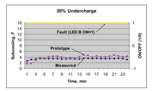
Figure 4-10 Subcooling Profile Along with ON/OFF Status for the 30% Undercharge Case.
