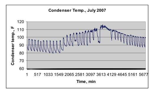
Figure 2-2 A Condenser Temperature Profile of an R-22 System.
