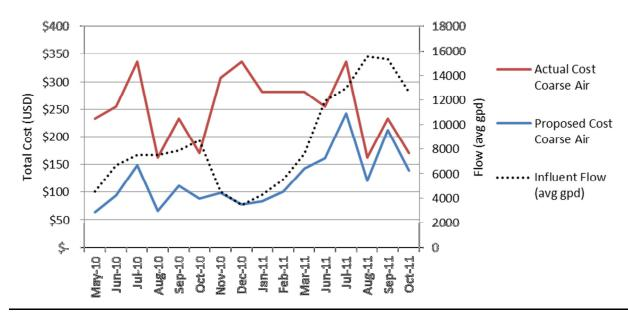
Figure 3. Proposed and actual cost of coarse aeration totalized by month over the study timeline. Proposed costs were determined based on the energy reduction potential of the proposed measures.
