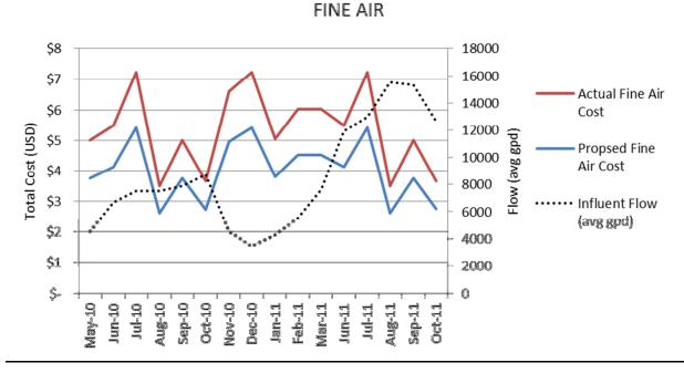
Figure 4. Proposed and actual cost of fine aeration totalized by month over the study timeline. Proposed costs were determined based on the energy reduction potential of the proposed measures.
