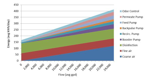
Figure 28. Comparison of the Specific Energy Consumption of the WTRS
