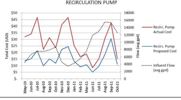
Figure 6. Proposed and actual cost of recirculation pump totalized by month over the study timeline. Proposed costs were determined based on the energy reduction potential of the proposed measures.
