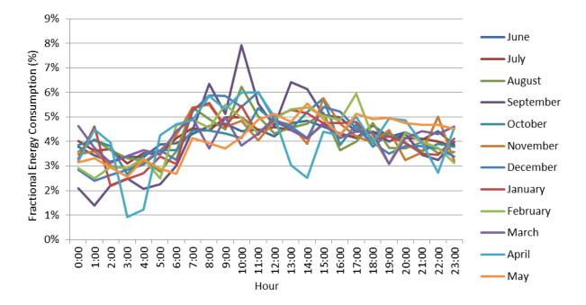
Figure 19. Hourly Power Consumption By The Booster Pump as a Fraction of Total Daily Power Consumption by The Booster Pump, for Each Monthly Average Day
