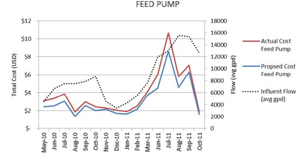
Figure 2. Proposed and actual cost of feed pump totalized by month over the study timeline. Proposed costs were determined based on the energy reduction potential of the proposed measures. Note the close correlation to the permeate pump costs.
