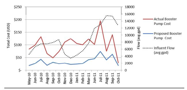
Figure 5. Proposed and actual cost of booster pump totalized by month over the study timeline. Proposed costs were determined based on the energy reduction potential of the proposed measures.
