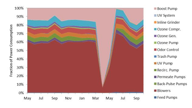
Figure 15. Fractional Power Consumption (%) of Each Component in the WTRS
