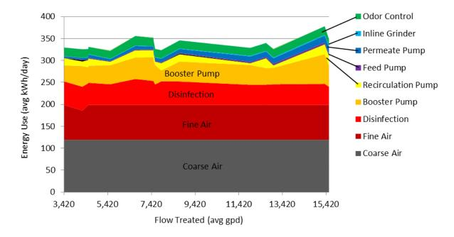
Additional power consumptions by the trash pump and back-pulse pump are negligible and are not shown.
