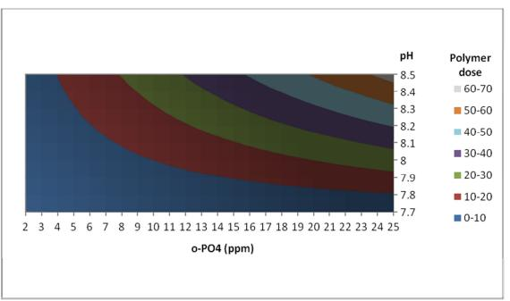
Figure 1: Chart demonstrating the relationship between orthophosphate concentration, pH, and the required polymer dose to prevent CaCO<sub>3</sub> and CaPO<sub>4</sub> scaling in an open recirculating cooling tower system.
