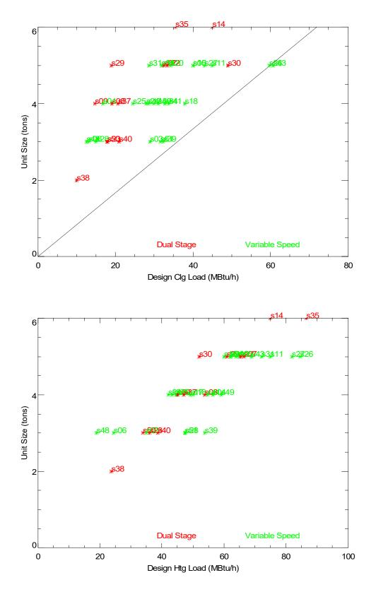
Figure A-2. Comparing Selected Heat Pump Unit Size to Design Heating and Cooling Loads
