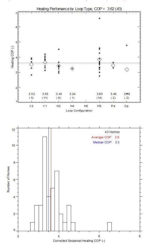
Figure 14. Distribution of Corrected Heating COPs—by Loop Type and for Total Sample
