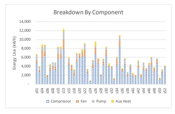
Figure 8. Breakdown of Annual Energy Use for GHP Systems by Site (data from Table 8)
