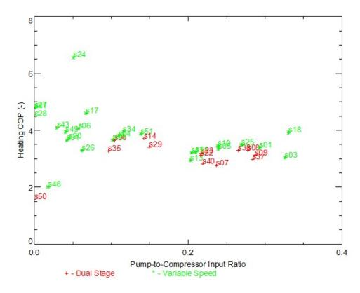
The on-site measurements from Site S8, a dual stage unit where the contractor installed two staged pumps in series, confirmed the relatively poor performance of this pumping arrangement and control strategy compared to variable speed operation. Table 12 shows the pumping power determined by the on-site measurements. The pump-to-compressor power ratio was 13% at high stage and 11% at low stage.
