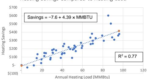
Heating Savings Compared to Heating Load
