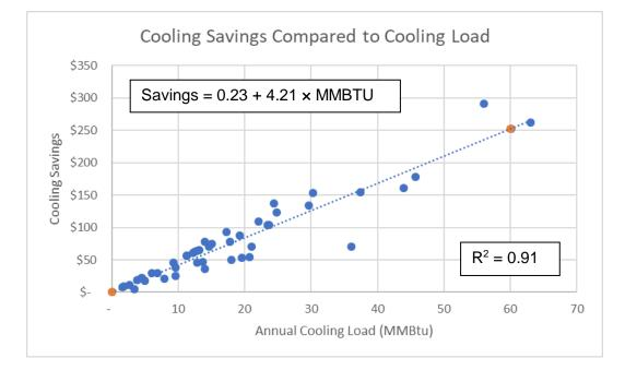
Figure 30. Trend of Cooling Cost Savings with Annual Cooling Load
