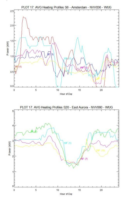
Figure 21. Winter Demand Profiles at Various Temperatures for S6 and S20
