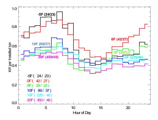
Figure 23. Average Winter Electric Demand Profiles at Various Outdoor Temperatures
