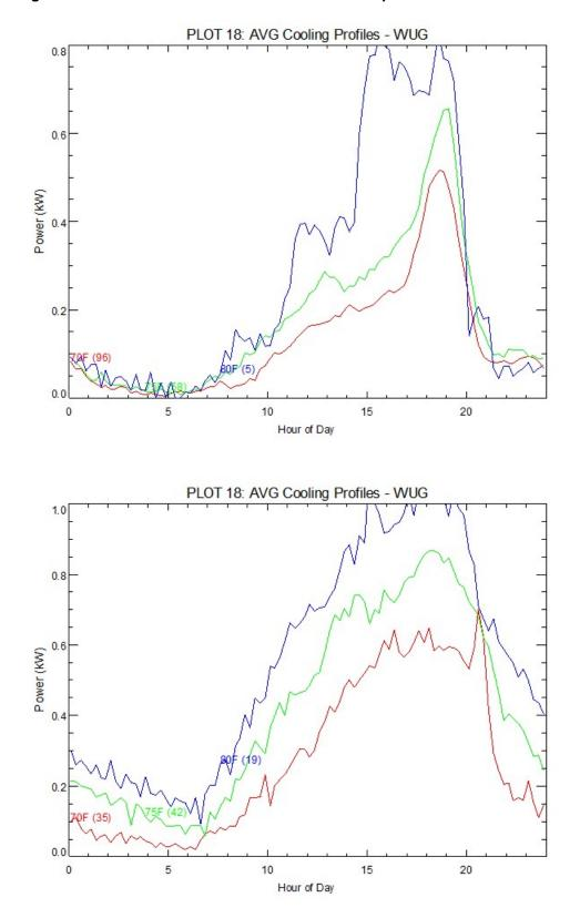
Figure 22. Summer Demand Profiles at Various Temperatures for S6 and S20
