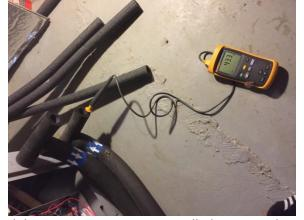
Fluke temperature sensor installed in petze plug for entering water
