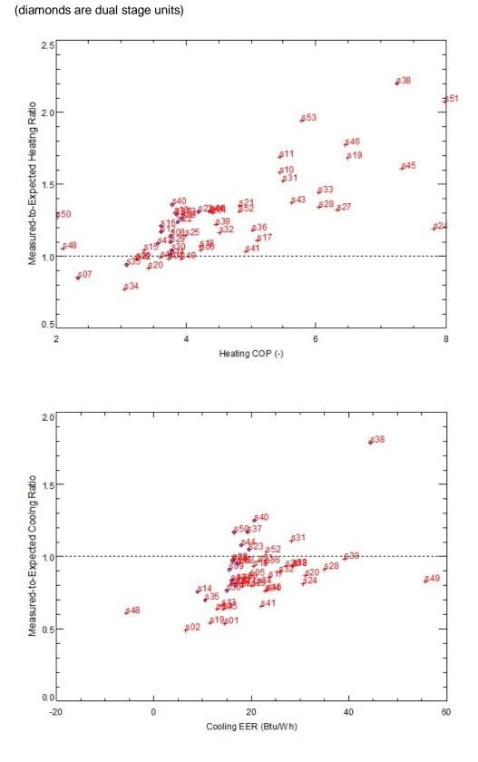
Figure 11. Comparing Measured-to-Expected Ratio for all Sites for Heating and Cooling
