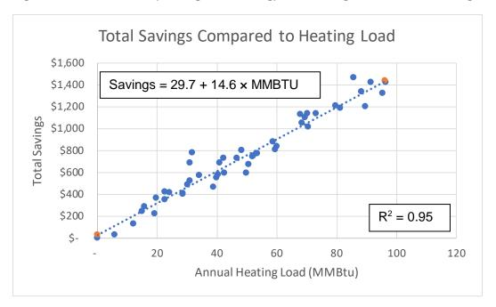
Figure 31. Trend of Total (Heating and Cooling) Cost Savings with Annual Heating Load
