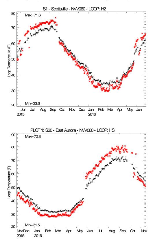
Figure 3. Daily Loop Temperatures at S1 (Horizontal Loop) and S20 (Horizontal Slinky Loop)
