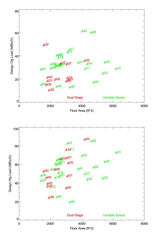
Figure A-1. Comparing Design Heating and Cooling Loads to House Floor Area
