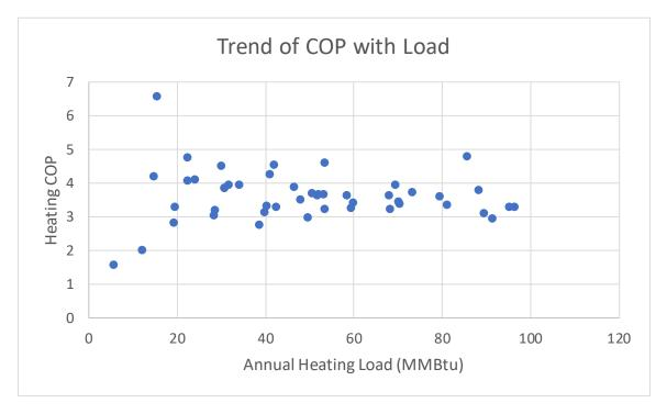
Figure 17. Trend of Seasonal Heating COP as a Function of Annual Heating Load
