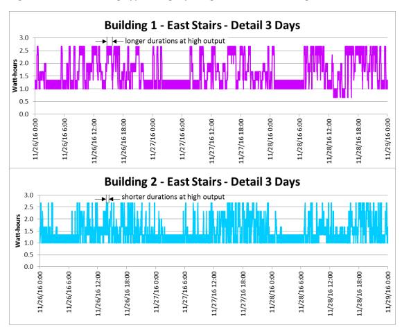
Figure 61. Detail Showing Typical Nightly Usage Patterns in Buildings 1 and 2
