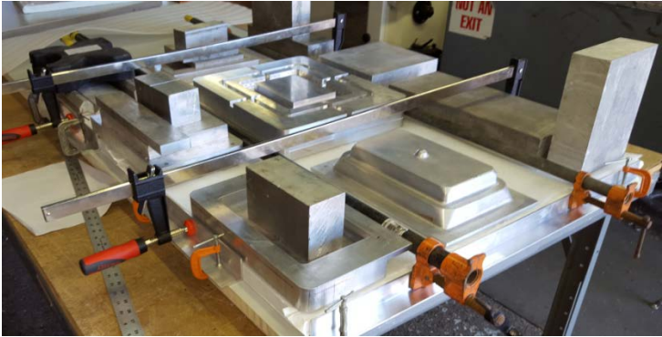
Figure 14. Weights added for z compression
