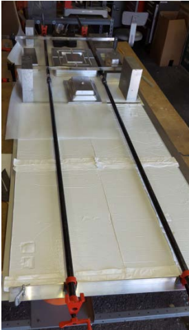
Figure 15. 2nd MAI-panel section with 1-inch polyisocyanurate spacer jigged
