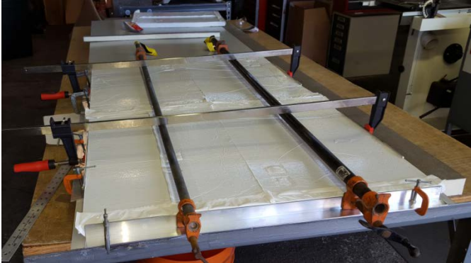
Figure 13. Four MAI panels clamped for x-y compression
