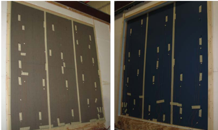
Figure 23. Meter-facing (left) and climate-facing (right) surfaces of the MAI composite test wall
