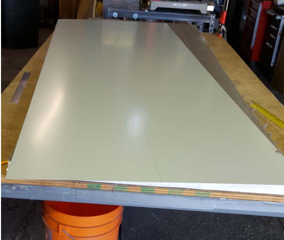
Figure 11. Metal sheet on 2-inch polyisocyanurate support
