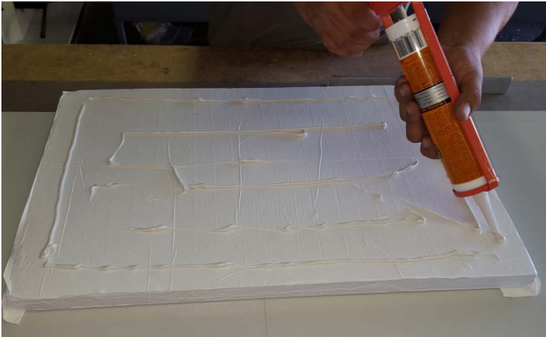
Figure 12. Adhesive being applied to MAI panels that are encased in membrane to minimize loss of vacuum
