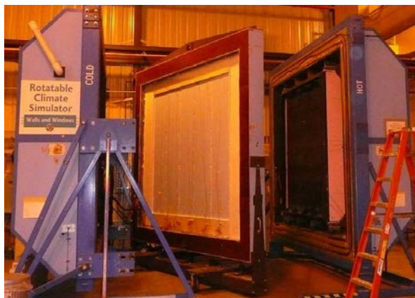
Figure 21. Rotatable Guarded Hot Box
