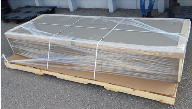
Figure 19. Three composite metal-MAI-polyisocyanurate panels on a pallet and ready for shipping to ORNL
