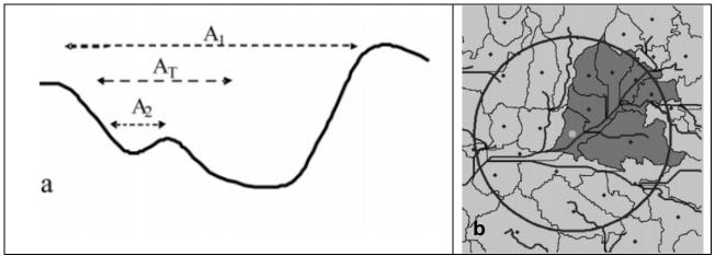
Figure 3-10. Illustration of catchment threshold size (panel a) and upstream search distance (panel b); creek drainages are also shown as dark lines in panel b.
