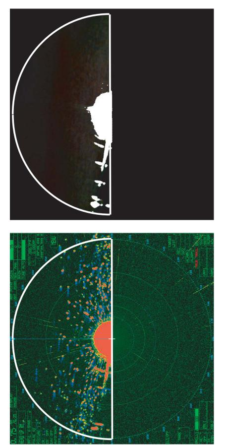
Figure 9. (Left) Data image from vertically oriented radar collected on 4 October 2008, 2244 EDT 10:44 PM). The thick white line graphically represents how NJAS's image processing software defines the sample area. (Right) Template generated by NJAS's image processing software for data collected on the same date as data image on the left. The template is used as a mask to remove stationary reflectors (i.e., main bang, ground clutter, see Figs. 3, 5, 6 for reference) from data images.
