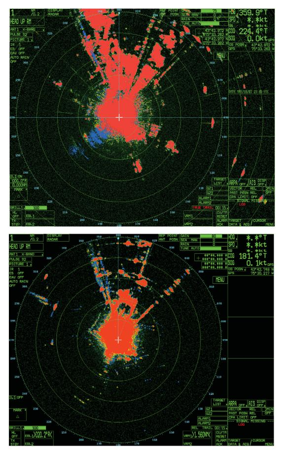
Figure 8. Image from horizontally-oriented radar showing backscatter of radar energy, or "ground clutter," within 1 nm of radar system on the Maple Ridge Wind Power Facility. (Upper) Radar's view of ground clutter at WTG 90, spring data collection site. (Lower) Radar's view of ground clutter at WTG 104, fall data collection site.
