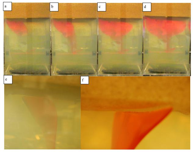
Figure 1: Stress barrier arresting fracture growth. Figure 1a-d top left to right: The weight of the sand creates a stress barrier in the uppermost layer of gelatin causing, (1a) a buoyant vegetable fracture to stop rising, (1b) preventing pressurized vertical propagation, (1c,d) and lateral fracture propagation; 1e,f bottom left and right: The fracture cannot push through the gelatin immediately below the sand and does not meet the sand layer above.
