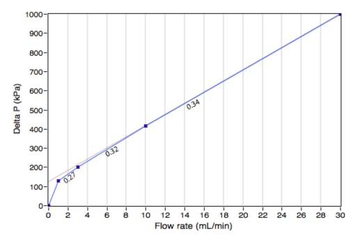
Figure 4: Sample results for relative permeability of  $CO_2$  in P3C alumina ceramic core at 20°C, 100 bars, DI water,  $k_{r_{2}CO2}=0.34$ . The blue line plots the flow rate vs. pressure drop data. The slope fit between adjacent data points provides the relative permeability, incorporating the capillary end effect.
