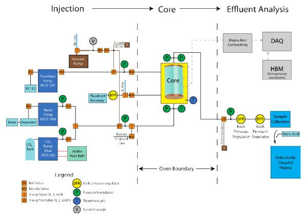
High Pressure Core Flooding Reactor
