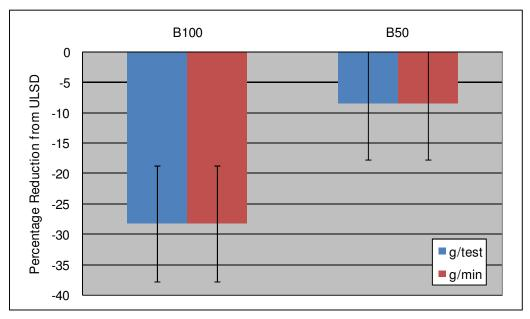
Figure 3-4. Reduction in NOx Emissions when Compared to ULSD Fuel
