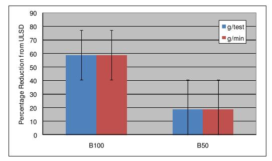
Figure 3-3. Reduction in CO Emissions when Compared to ULSD Fuel
