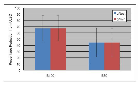
Figure 3-1. Reduction in PM Emissions when Compared to ULSD Fuel
