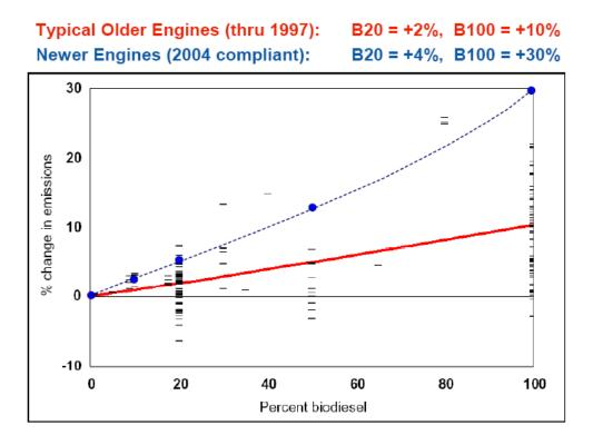
Figure 3-6. Influence of Engine Age on Biodiesel's Effect on NOx Emissions
