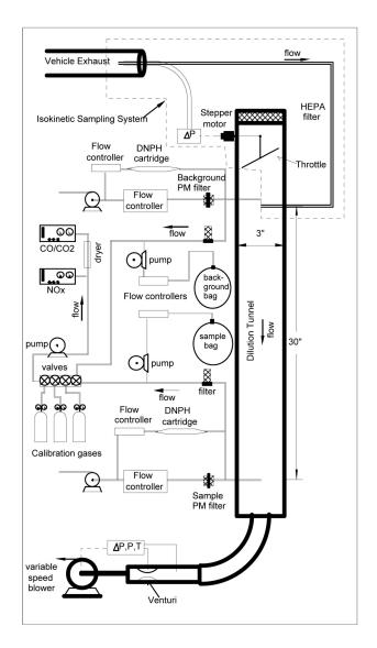
Figure 2-2. Diagram of the RAVEM System (courtesy of EF&EE)
