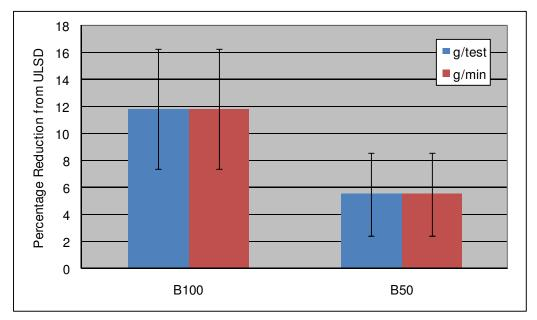
Figure 3-2. Reduction in CO<sub>2</sub> Emissions when Compared to ULSD Fuel
