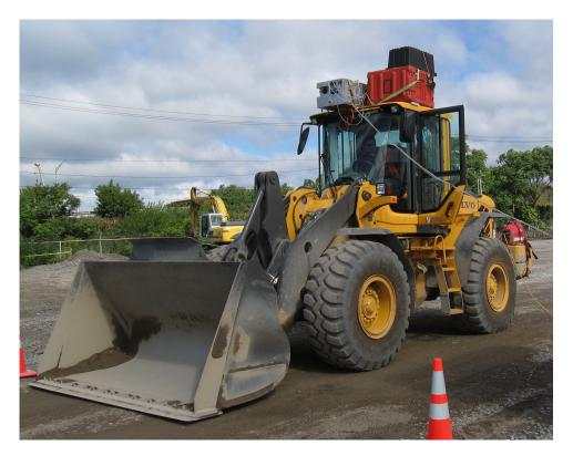
Figure 2-1. Volvo L90F Instrumented for In-Use Testing
