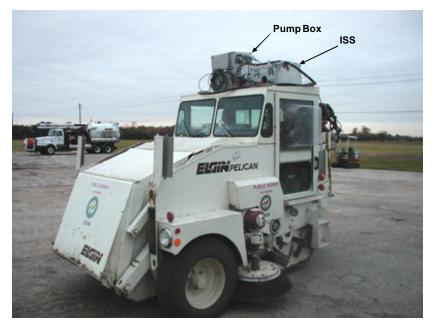
Figure 6-3. Example ISS and Pump Box Installation on a Sweeper (photo courtesy of Environment Canada)
