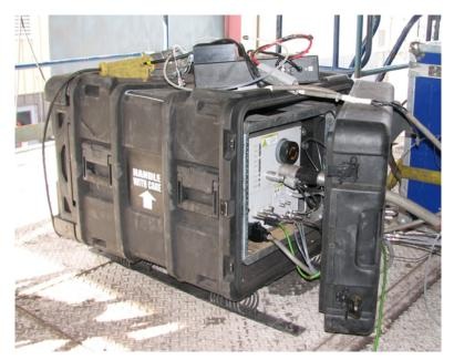
Figure 6-1. Example PEMS Installation
