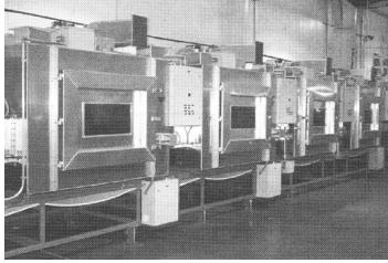
Figure 51. Modular Conveyor Oven
