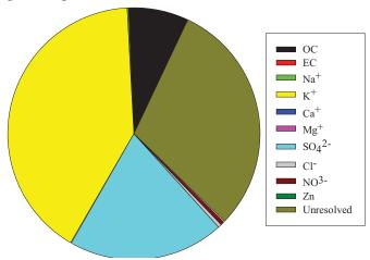
**Figure ES2.** Pie chart of fine PM composition from stack emission of Walker Center boiler when burning wood pellets.
