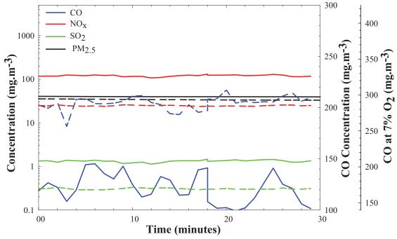
**Figure 6.** Concentration of criteria pollutants (CO, NO<sub>x</sub>, SO<sub>2</sub> and PM<sub>2.5</sub>) during steady state operation of 150 kW boiler (at full load). Dashed lines indicate data for wood pellets (Walker Center boiler) and solid line indicate data for wood chips (ACT Bioenergy boiler).
