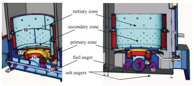
**Figure 1**. Detailed view of fuel feed auger, ash augers, and combustion zones of a Hamont Boiler. (from Hamont European Operating Manual for CATfire 150-500 kW Wood Boilers).
