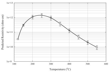
Figure 13. Ash resistivity as predicted from the Bickelhaupt's model
