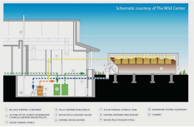
**Figure 2.** Schematics of commercial size pellet boiler with solar thermal system at The Wild Center. Obtained from www.wildcenter.org.
