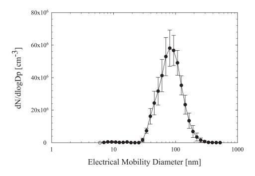
**Figure 5.** Ultrafine particle number size distribution during steady state of the boiler at Walker Center, Clarkson University. Error bars are one standard deviation.
