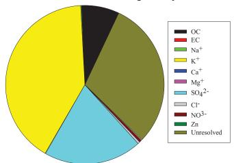
**Figure 4.** Pie chart of fine PM composition from stack emission of Walker Center boiler when burning wood pellets.
