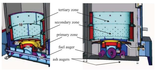
**Figure ES1**. Detailed view of fuel feed auger, ash augers, and combustion zones of a Hamont Boiler. (from Hamont European Operating Manual for CATfire 150-500 kW Wood Boilers).
