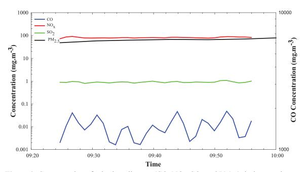
**Figure 9.** Concentration of criteria pollutants (CO,  $NO_x$ ,  $SO_2$  and  $PM_{2.5}$ ) during steady state operation of 500 kW boiler (at full load).
