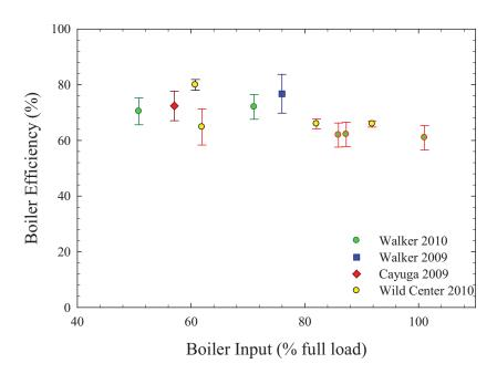
**Figure 11.** Thermal efficiency of the Walker Center, ACT Bioenergy and Wild Center boilers using the gross calorific value with 95% confidence intervals. The data points with red edges indicate data when the boiler was manipulated to run at 100% of the selected feed rate.
