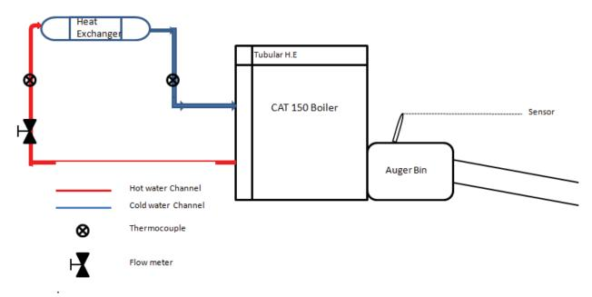
Figure 3. Illustration of boiler piping with approximate location of thermocouple and flowmeter.
