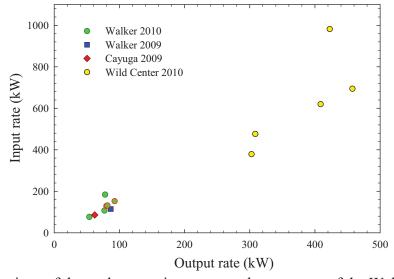
**Figure 12.** Comparison of thermal energy input rate and output rate of the Walker Center, ACT Bioenergy and Wild Center boilers (input rate calculated using the gross calorific value). The data points with red edges indicate data when the boiler was manipulated to run at 100% of the selected feed rate.
