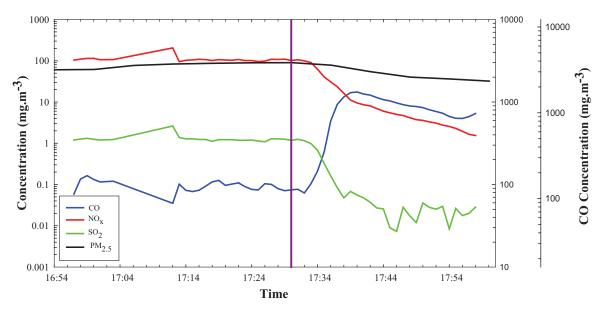
**Figure 7.** Concentration of criteria pollutants (CO, NO<sub>x</sub>, SO<sub>2</sub> and PM<sub>2.5</sub>) during shutdown of ACT Bioenergy boiler buring wood chips. Boiler shutdown was initiated at 17:30 hrs.
