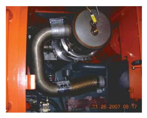
Figure 3-12. Left-Side View of the ECS DPF Installed on a Case 821 Rubber Tire Loader
