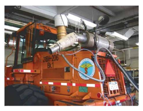
Figure 3-11. CleanAIR Systems PDPF Installed on a Case 821 Rubber Tire Loader and Instrumented for In-Use Emissions Testing
