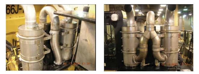
Figure 3-9. Front (left) and Rear (right) View of the Huss ADPF Dual Filter Retrofit Installed on a CAT D400 Dump Truck
