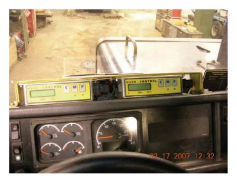
Figure 3-10. In-Cab Display of Huss ADPF Control Modules Installed in the CAT D400 Dump Truck
