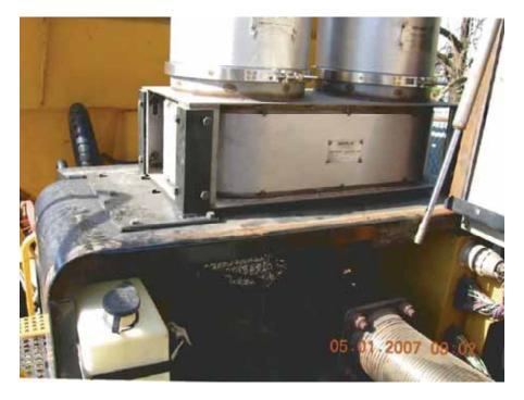
Figure 3-8. Front View of the Johnson Matthey DPF Mounting Arrangement
