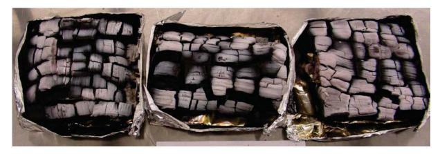
Figure 3-10. Final Char for Ash Wood Sample.
