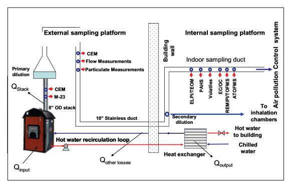
Figure 6. Test System for Wood-Fired Hydronic Heaters.
