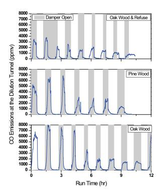
Figure 12. Typical CO Concentration Traces from the Dilution Tunnel for the Conventional, Single Stage HH Unit.
