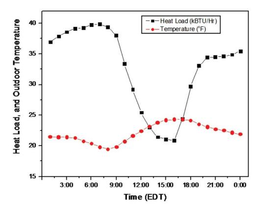
Figure 5. Syracuse, New York Area Heat Load Profile for the First Two Weeks of January.
