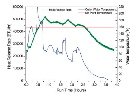
Figure 9. Heat Release Rate from the U.S. Two Stage Downdraft Burner Unit with Thermal Storage.
