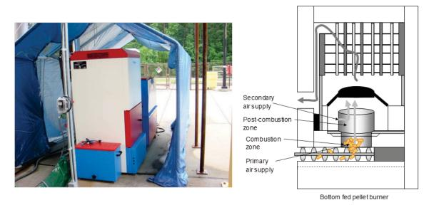
Figure 3. The European Two Stage Pellet Burner and Illustration of a Bottom-Fed Pellet Combustion Unit.
