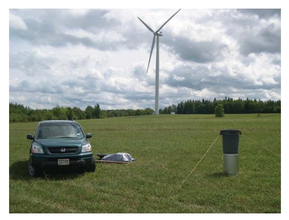
Figure 3. Avian acoustic recording station. Skyward-facing microphone is in gray cylinder. Recording gear and batteries are under plastic tarp.
