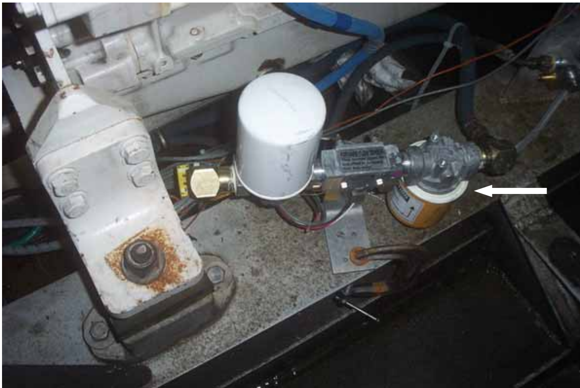
Figure 2.5. FloScan Fuel Supply Meter, MV FATHER MYCHAL JUDGE Main Engine.
