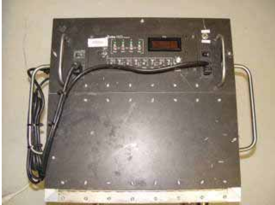
Figure 2.10. Flow Control for Sample and Dilution (top).
