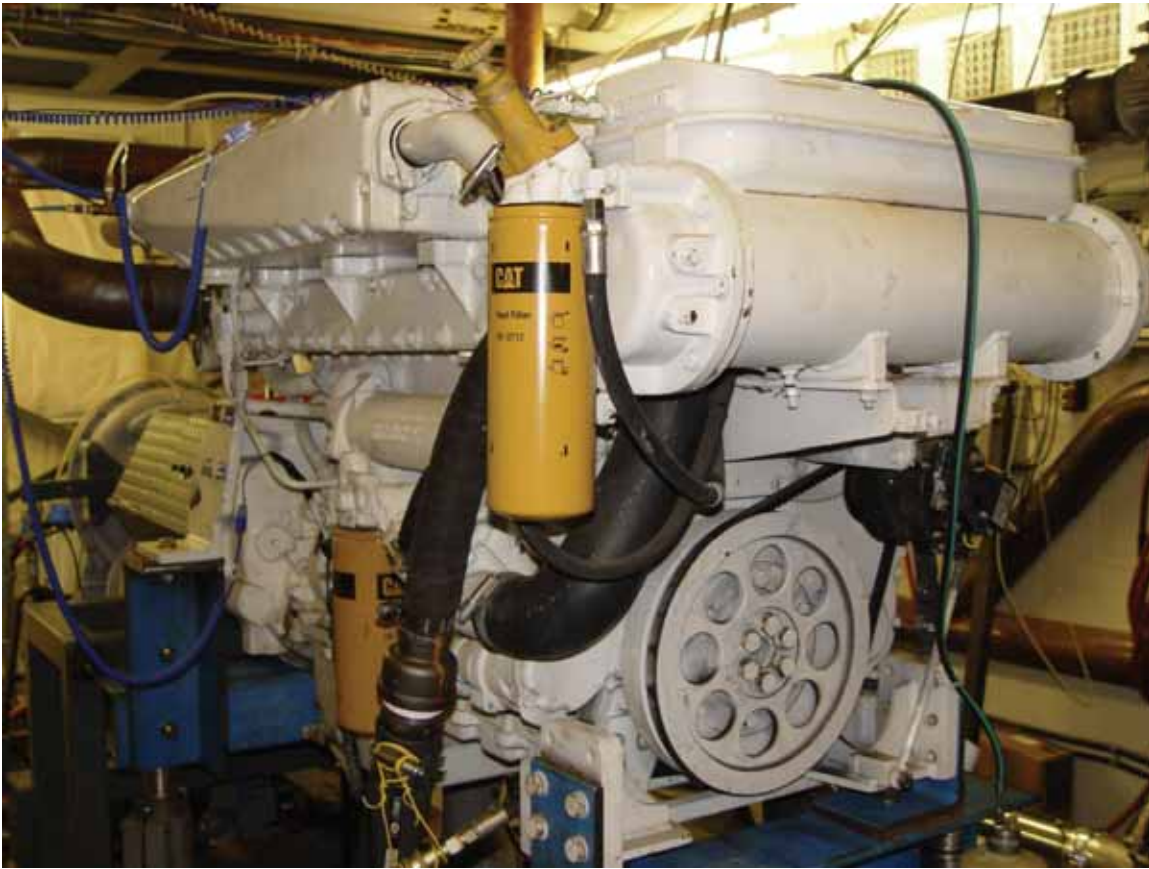
Figure 4.1. 1994 Caterpillar 3176 600hp Marine Engine.
