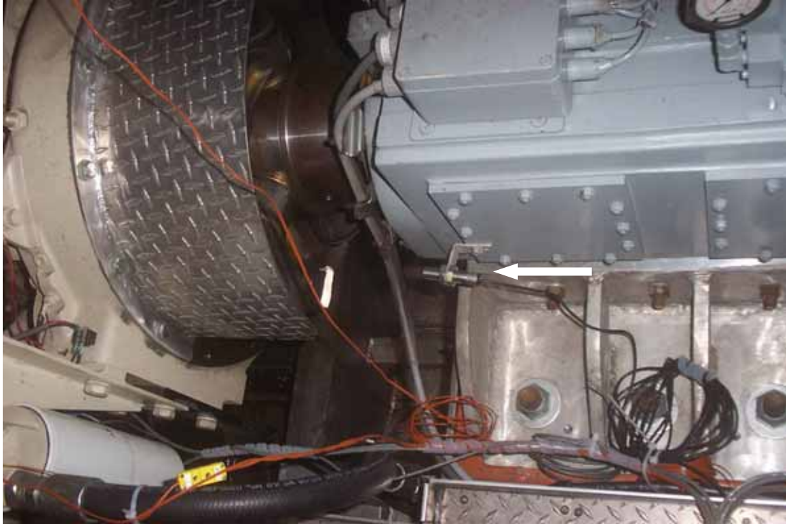
Figure 2.4. Engine RPM Sensor and Reflective Tape, MV SEASTREAK WALL STREET Port Aft Main Engine.
