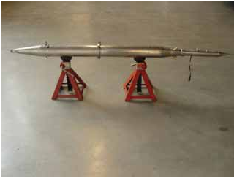
Figure 2.7. Mini-Dilution Tunnel (Total Length 82 inches).
