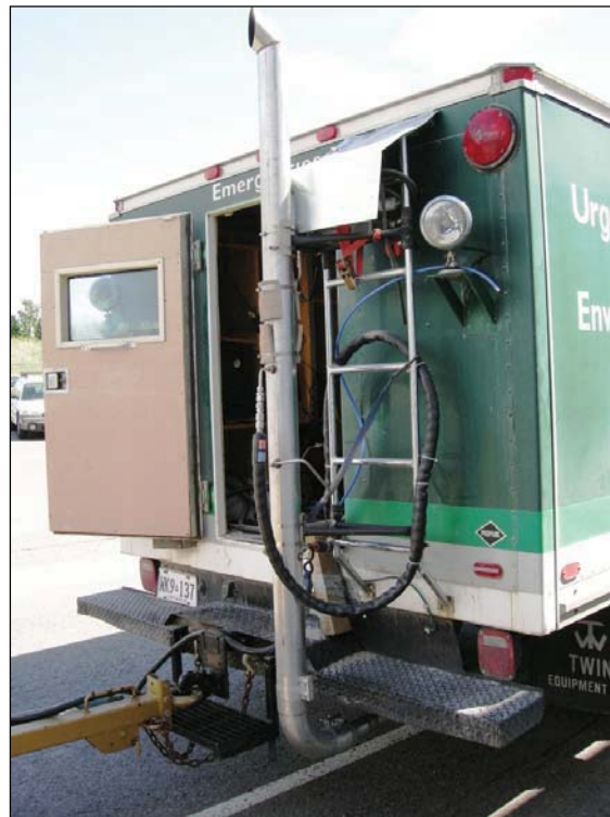
Figure 3-7. Routing of the Exhaust Tube for Installation of PM PEMS Equipment
