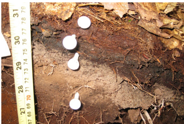
Figure 4. Soil pits were excavated at each study plot to collect samples from each horizon. (Source: E&S)
