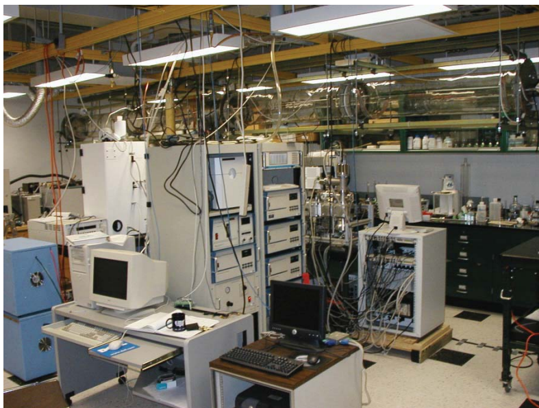
Figure C-1. Aerosol Generation, Calibration and Research Facility.
