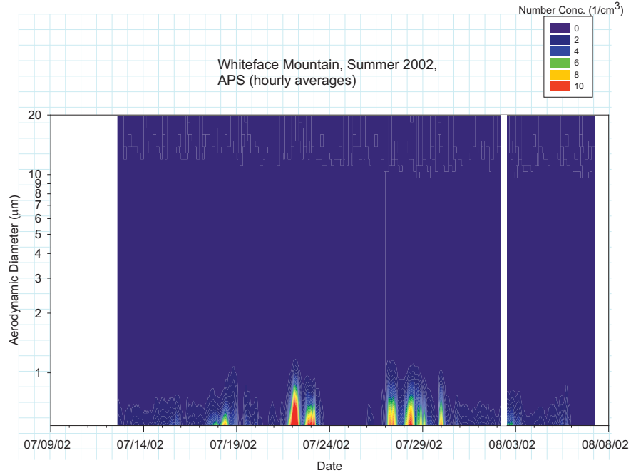
Figure 6.1-30. Time series of hourly particle size distributions from the APS during the WFM2002 summer campaign.
