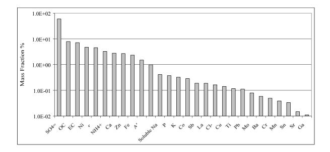
Figure 5-1b. Primary Emissions Speciation Profile for Oil Operation (Delta).
