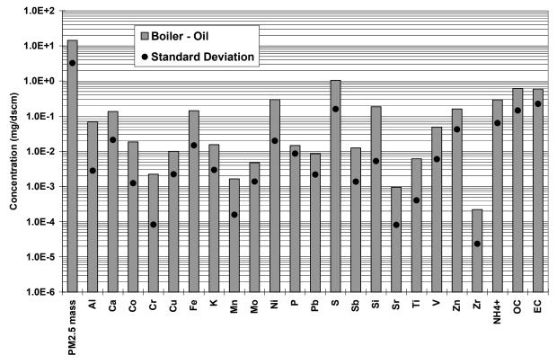
Figure 7-1b. Mass Speciation - DS Ambient and Stack Samples (Delta - Oil).
