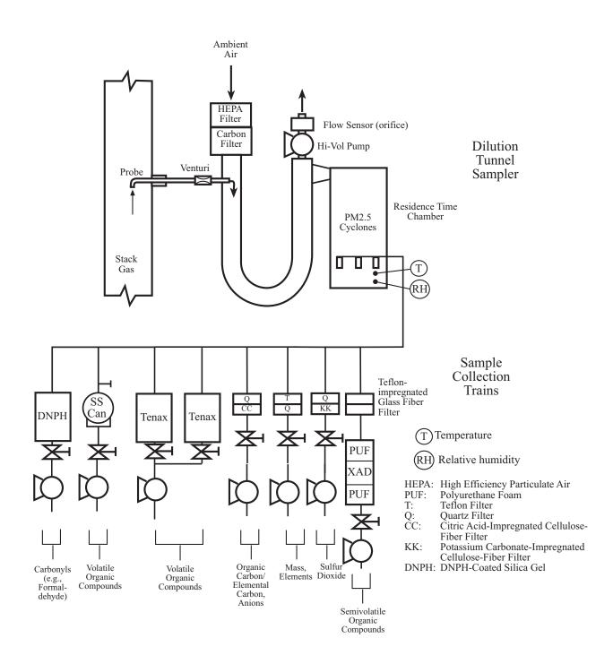
Figure 3-2. Dilution Sampler System.
