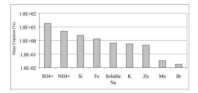
Figure 5-1a. Primary Emissions Speciation Profile for Natural Gas Operation (Delta).
