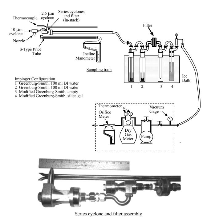
Figure 3-2. PM10/PM2.5 Train Configuration for Method PRE-4/202.
