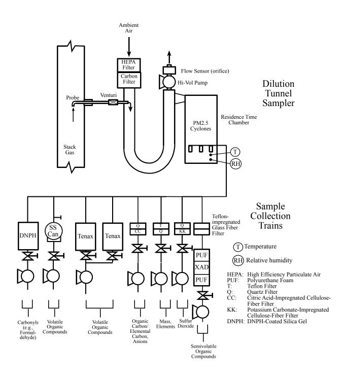
Figure 3-5. Dilution Sampling System.
