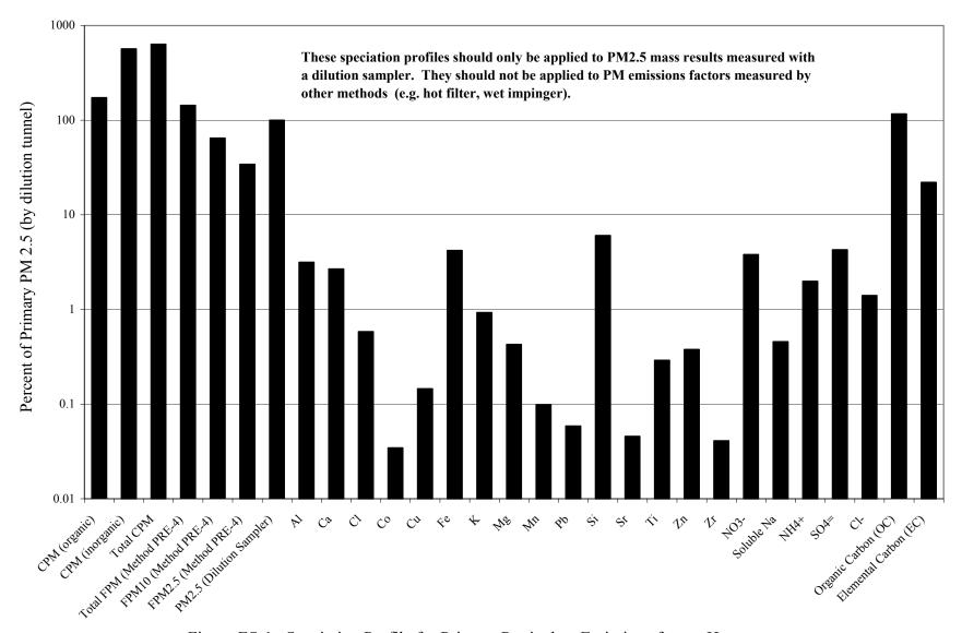
Figure ES-1. Speciation Profile for Primary Particulate Emissions from a Heater.
