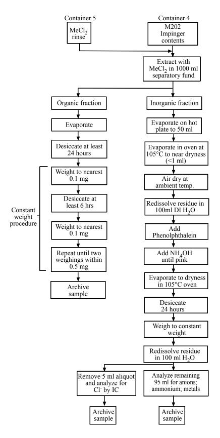
Figure 3-3. Modified Method 202 Sample Analysis Procedure.
