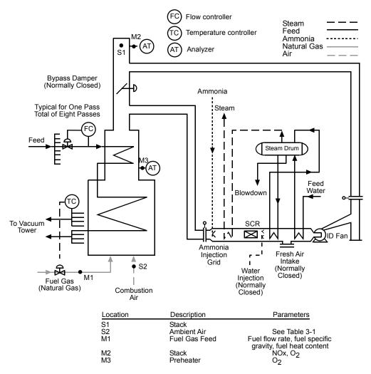
Figure 2-1. Gas-Fired Heater Process Overview.
