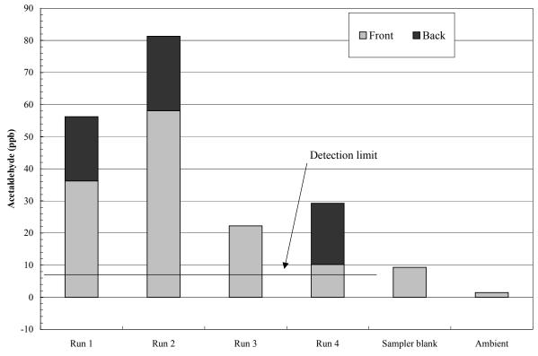
Figure 7-4. Sampler Blank-Corrected Acetaldehyde Concentrations (Site Charlie).
