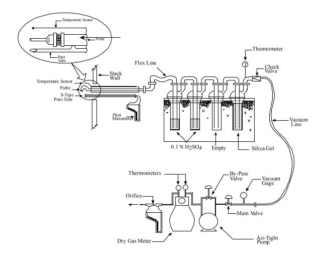
Figure 3-4. Ammonia Sample Train Configuration for SCAQMD Method 207.1.
