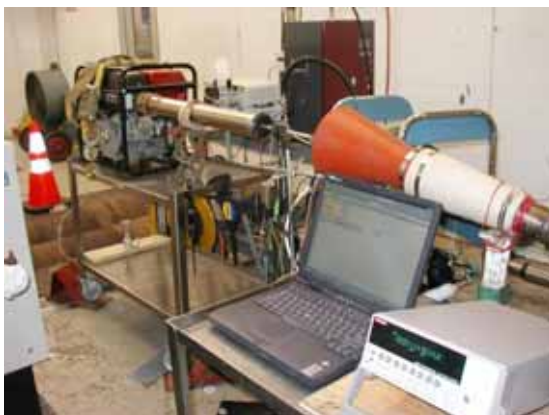
Figure 2.4. (a) A picture of experimental set-up for chemion measurements, and (b) time series of imposed voltage and measured current ( I ) in the exhaust of a Honda gasoline generator.
