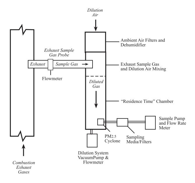
Figure 2. Dilution sampling system schematic
