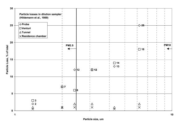
Figure 2-4. Dilution Sampler Particle Losses (from Hildemann et al., 1989).
