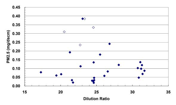
Figure 2-30. PM2.5 versus Dilution Ratio (All Gas-Fired Sites, DRI and Compact Samplers).
