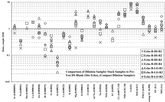
Notes: (1) Number in parentheses in x-axis labels indicates average stack sample concentration, mg/dscm; (2) ND in  $\vec{x}$ -axis labels indicates substance not detected in blank, detection limit used for ratio.
