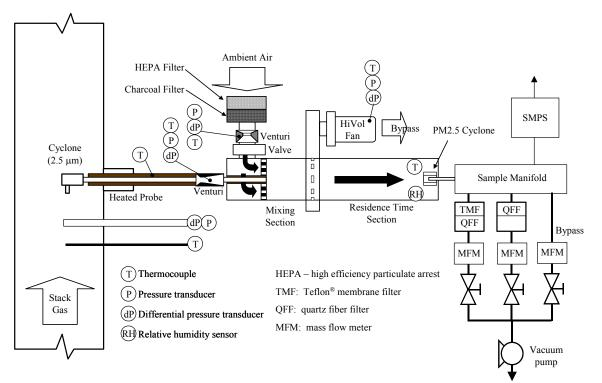
Figure 2-9. Compact Dilution Sampler.
