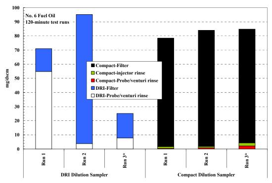
\*Run 3 invalid due to abnormal combustion, run terminated after 53 minutes.
