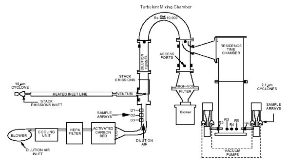
Figure 2-6. U.S. EPA Dilution Sampler (Dayton and Bursey, 2001).
