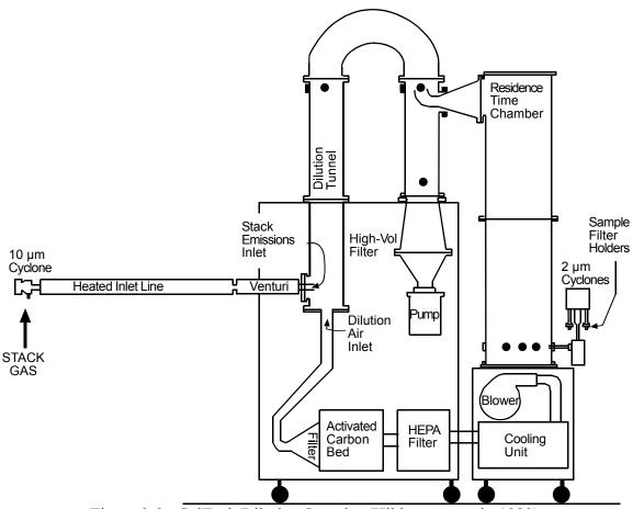
Figure 2-3. CalTech Dilution Sampler (Hildemann et al., 1989).
