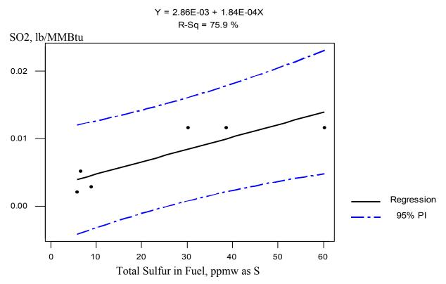
Figure 3-5. Correlation of SO<sub>2</sub> with Fuel Sulfur for Gas-Fired Boilers.
