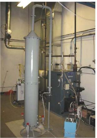
Figure 2-7. CANMET Dilution Sampler Version 3 (Lee et al., 2003).
