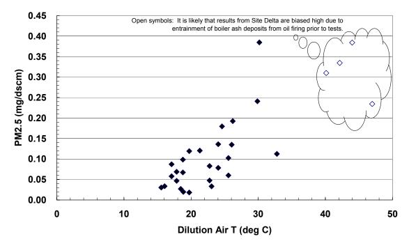
Figure 2-28. PM2.5 versus Dilution Air Temperature (All Gas-Fired Sites).
