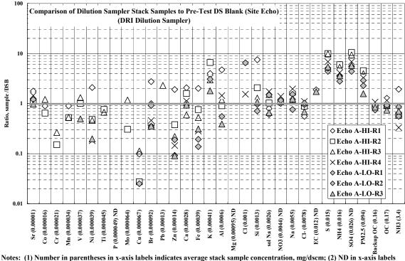
Notes: (1) Number in parentheses in x-axis labels indicates average stack sample concentration, mg/dscm; (2) ND in x-axis la indicates substance not detected in blank, detection limit used for ratio.
