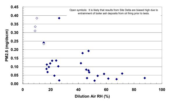
Figure 2-27. PM2.5 versus Dilution Air Relative Humidity (All Gas-Fired Sites). Temperature
