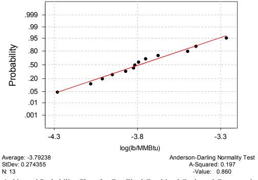
Figure 3-4. Normal Probability Chart for Gas-Fired Combined Cycle and Cogeneration Power Plant PM2.5 Mass Results.
