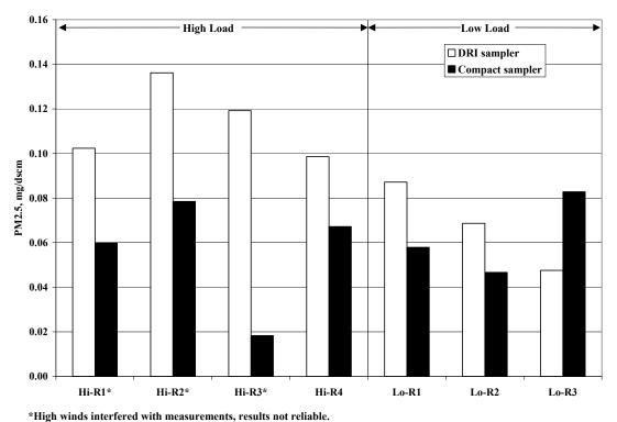
Figure 2-13. Comparison of DRI and Compact Dilution Sampler PM2.5 Results for a Natural Gas-Fired Combined Cycle Power Plant with Oxidation Catalyst and SCR (England et al., 2004).
