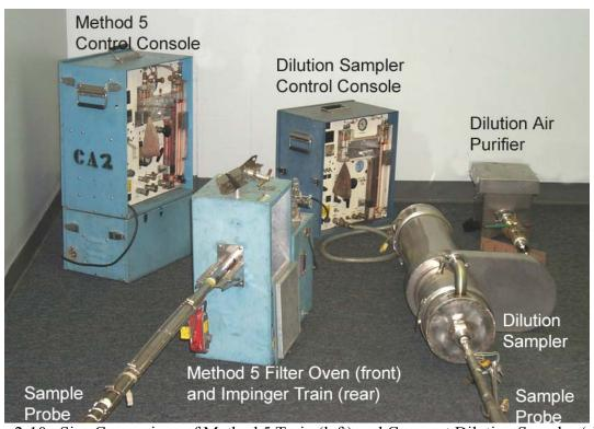
Figure 2-10. Size Comparison of Method 5 Train (left) and Compact Dilution Sampler (right).
