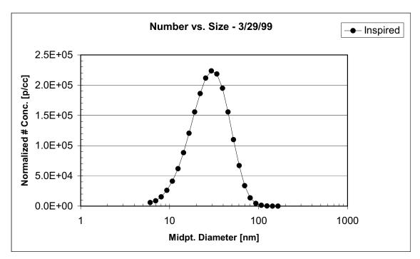
Figure 2-2. Size distribution, by number, of ultrafine carbon particles generated for inhalation.
