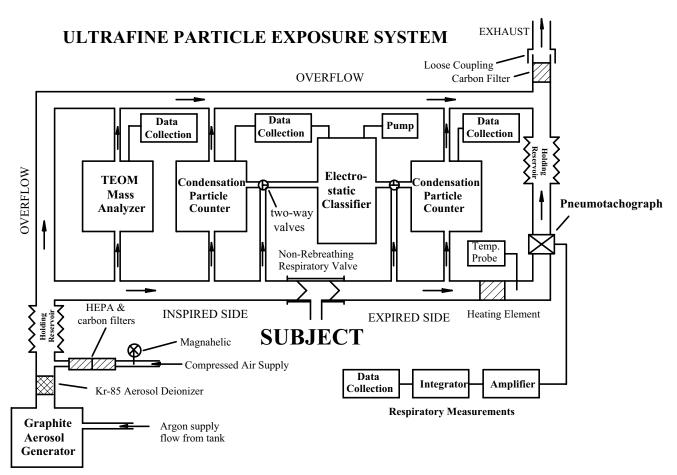
**Figure 2-1.** Ultrafine particle generation and exposure system. "Subject" indicates the position of the volunteer being exposed, breathing through a mouthpiece. The non-rebreathing valves direct airflow in a single pass from the holding reservoir on the inspiratory side toward the expiratory holding reservoir and exhaust. Positions of monitoring equipment and ports are indicated; see Table 1 for equipment sources.
