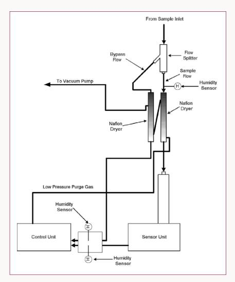
**Figure 1.** Schematic of the SES equipped TEOM monitor
