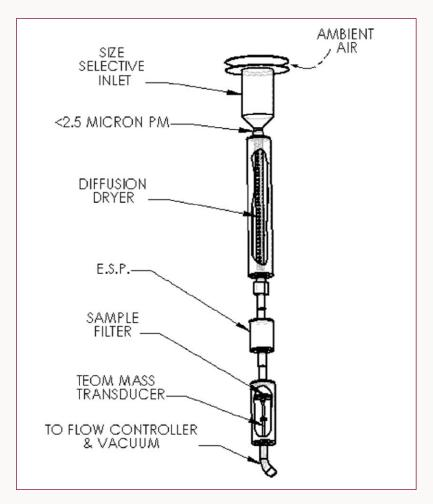
**Figure 2.** Schematic of the Differential TEOM monitor
