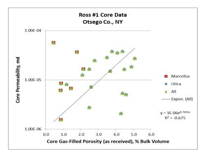
Figure 18: Ross #1; Cross-Plot of Core Permeability and 'Gas-Filled' Core Porosity
