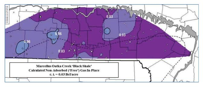
Figure B-4: Marcellus Oatka Creek 'Black Shale' Calculated Non-Adsorbed ('Free') Gas In-Place, Bcf/ac
