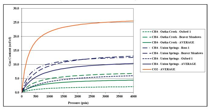
Figure 11: Marcellus CH<sub>4</sub> and CO<sub>2</sub> Adsorption Isotherms
