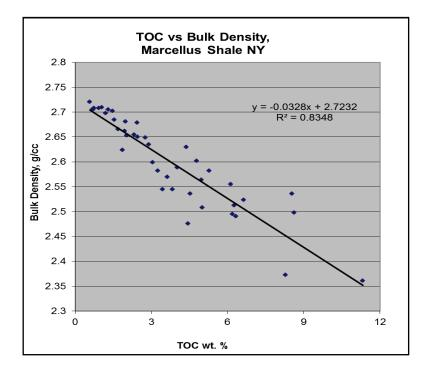
Figure 13: TOC vs Bulk Density for Marcellus Shale
