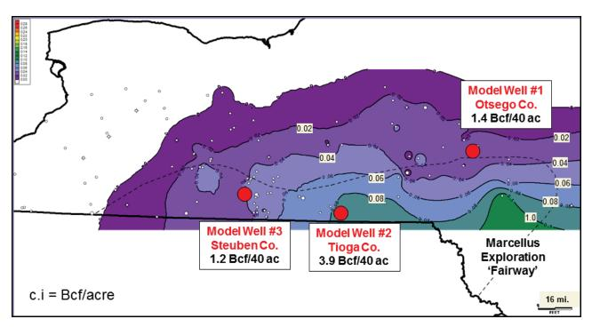
Figure 17: Marcellus Union Springs – Calculated Maximum CO2 Storage Capacity Replacing Non-Adsorbed Methane in Effective Porosity, Bcf/ac
