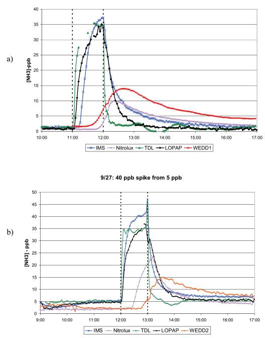
Figure 1-2. Instrument responses to two 40 ppb spike calibrations. a) [NH<sub>3</sub>] is increased from zero to 40 ppb for one hour, then back to zero. b) [NH<sub>3</sub>] is increased from 5 ppb to 40 ppb for one hour, then back to 5 ppb.
