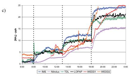
**Instrument responses** to three different calibration exercises. a) The exercise starts with scrubbed "zero air", followed by 20 ppb for 15 hours, zero air for one hour and 20 ppb for two hours. b) Starting from zero air, the NH<sub>3</sub> concentration is raised to 5 ppb for 8 hours, then to 10 ppb overnight. c) This exercise starts with zero air, followed by 5 hours of 5 ppb ammonia, 5 hours of 10 ppb NH<sub>3</sub>, and 20 ppb NH<sub>3</sub> overnight.
