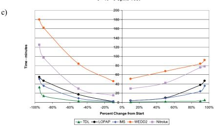
**Figure 1-4. Instrument** response times to step changes in the ammonia concentrations supplied by the calibration system. a) A zero to 20 ppb step performed as part of a calibration exercise on 9/19/2005. b) Rise and fall times for the zero to 40 ppb and 40 to zero ppb steps that made up the September 26 spike test. c) Rise and fall times for the 5 to 40 ppb and 40 to 5 ppb steps that made up the September 27 spike test.
