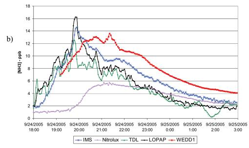
Figure 1-3. Instrument responses to ambient air sampled through the heated sample manifold for two periods are shown. a) Data from September 18 and 19, 2005. b) Data from September 24 and 25, 2005.
