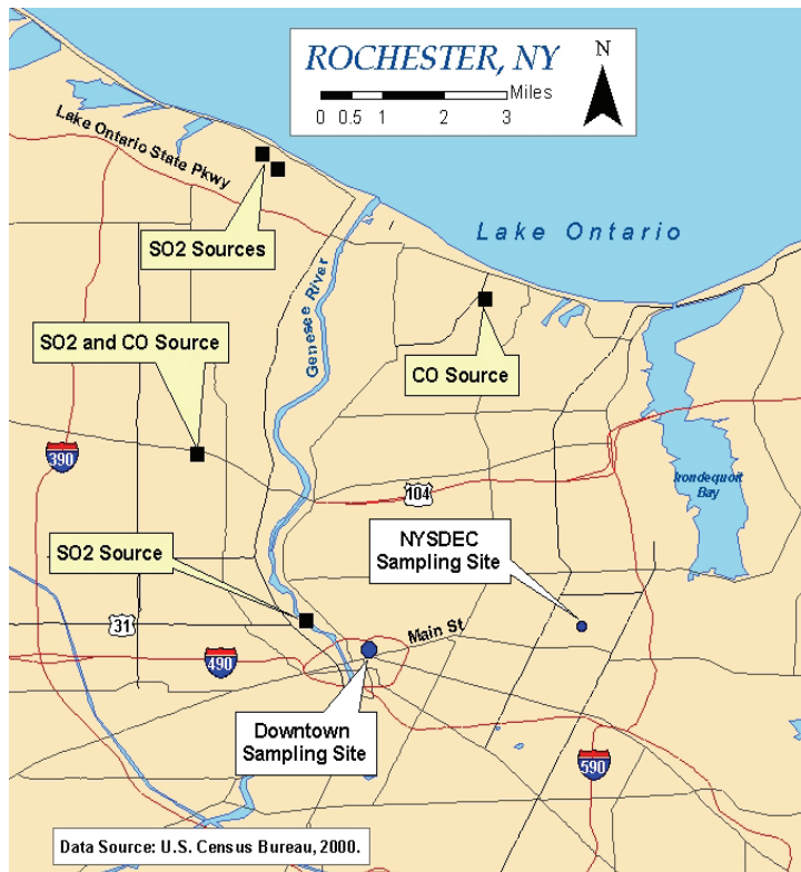
Figure 1. Locations of sampling sites and major local stationary sources as listed in the EPA point source emissions inventory .
