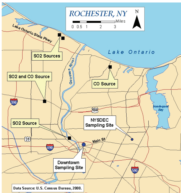
Figure S1. Locations of sampling sites and major local stationary sources as listed in the EPA point source emissions inventory.
