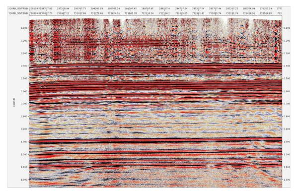
Figure 17: Line 101 after migration and with post-migration processing. Correcting for residual statics has flattened many of the reflectors. West is on the left.
