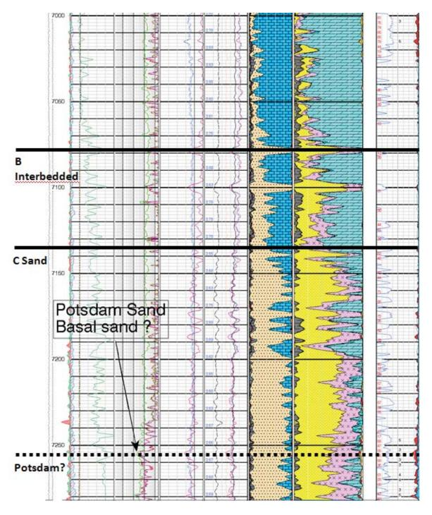
Figure 9: Miller 2 well ELAN analysis for the B Dolomite, B Interbedded, and C Sand Members of the Galway Formation and possibly the Potsdam Formation (7000-7300 feet).
