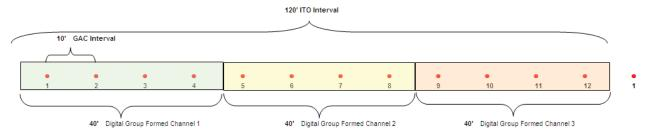
Figure A.3 GAC - IDF array scheme
