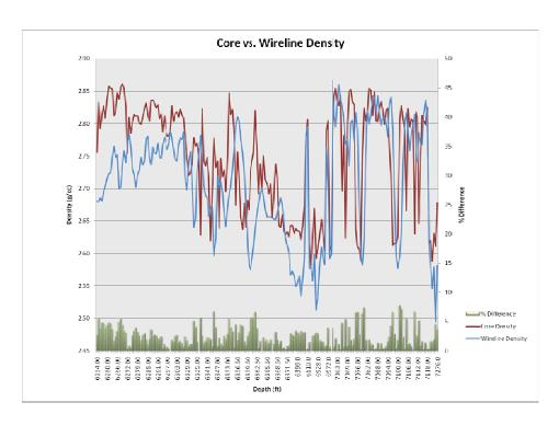
Figure 6-6. Graph Showing Measured Core Density Versus Measured Wireline Density for Miller #2 (in g/cm³) and the Percent Difference between the Two Curves
