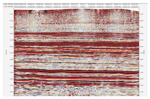
Figure 18: Line 301 after migration and with post-migration processing. Correcting for residual statics has flattened many of the reflectors. North is on the left.
