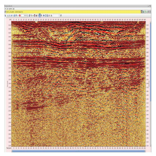
Figure A.16 - Field Brute Stack - Line 301
