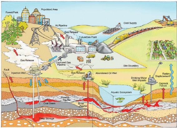
Figure 1 - Conceptual Model for Carbon Capture and Sequestration process. (Taken from DOE 2007)
