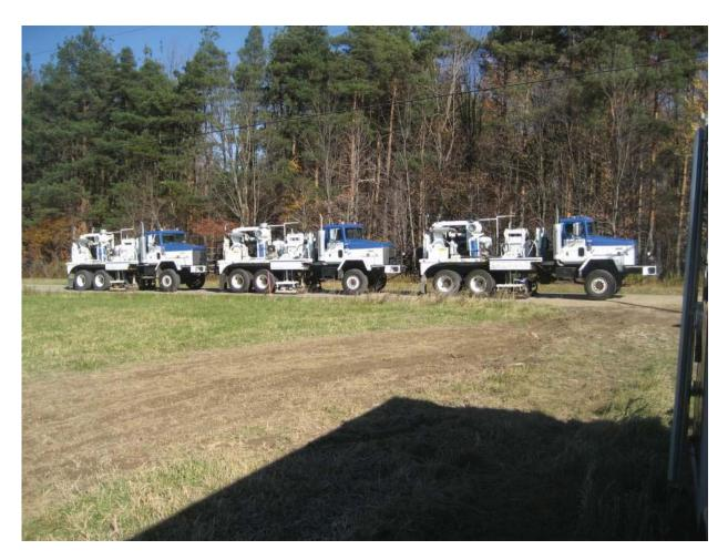
Figure 11: View of prospect area with vibrator trucks
