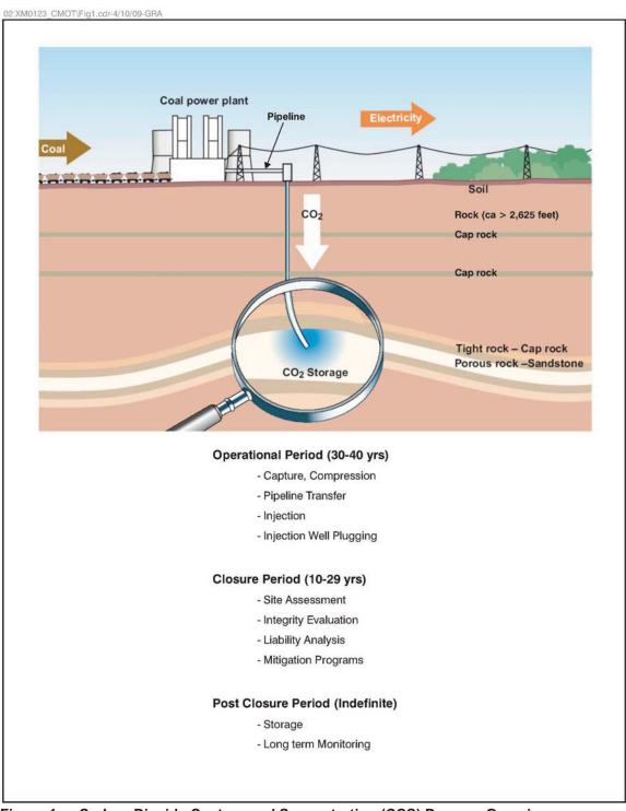
Figure 1 Carbon Dioxide Capture and Sequestration (CCS) Process Overview
