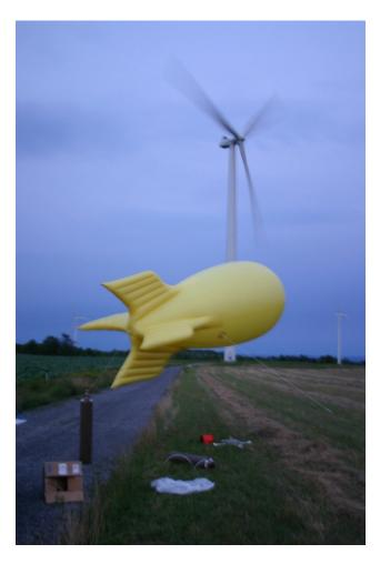
Figure 45. Deployment of tethered blimp at Maple Ridge Wind Farm
