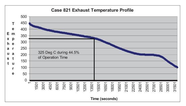
Figure 0-5. Case 821 Rubber Tire Loader, Temperature Data Logging
