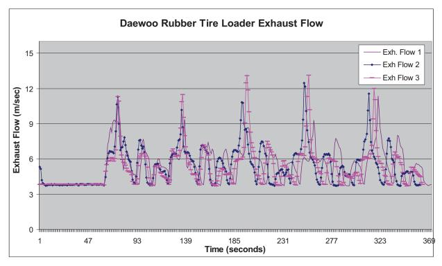
Figure 3-6. Daewoo Mega 200 Rubber Tire Loader, Exhaust Flow Data Logging
