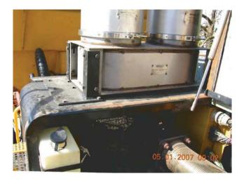
Figure 4-11. Front View of the Johnson Matthey DPF Mounting Arrangement
