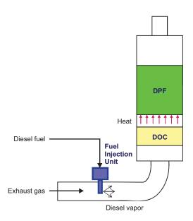
Figure 4-12. Filter with Catalytic Combustion of Fuel
