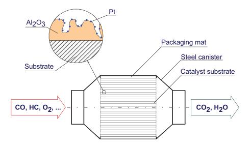
Figure 4-22. Schematic of Diesel Oxidation Catalyst
