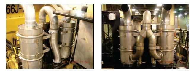
Figure 4-15. Front (left) and Rear (right) View of the Huss ADPF Dual Filter Retrofit Installed on a CAT D400 Dump Truck
