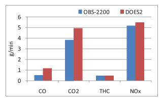
Figure 4-23: Pre-CleanAIR PDPF Emissions Results from the OBS-2200 and the DOES2
