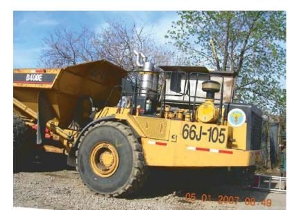
Figure 4-10. Johnson-Matthey DPF installed on a CAT D400 Dump Truck
