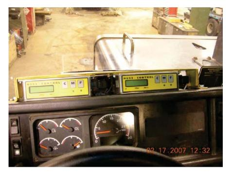
Figure 4-16. In-Cab Display of Huss ADPF Control Modules Installed in the CAT D400 Dump Truck
