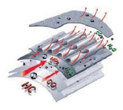
Figure 4-18. "PM Filter Catalyst" Honeycomb Substrate (Emitec)
