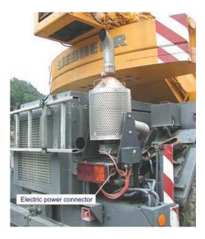
Figure 4-13. Shore Power Regenerated Filter on Construction Machinery (Switzerland)
