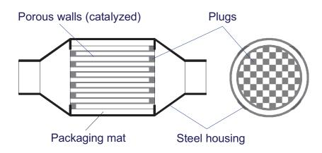
Figure 4-1. Catalyzed Diesel Particulate Filter
