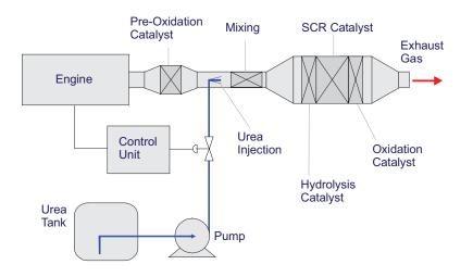
Figure 4-20. Generic Schematic of Urea-SCR System (Open Loop Control)
