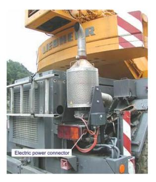
**Figure 4-7. Shore Power Regenerated Filter on Construction Machinery (Switzerland)** To perform the regeneration, the driver/operator must park the vehicle near a power outlet, connect the DPF system to the power, and initiate the regeneration sequence. The regeneration is usually conducted
