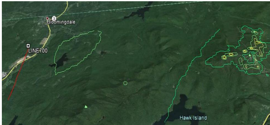
Figure 6-7. Dry and total Hg2 deposition from a 1000m source at SW edge of the Catskills grid
