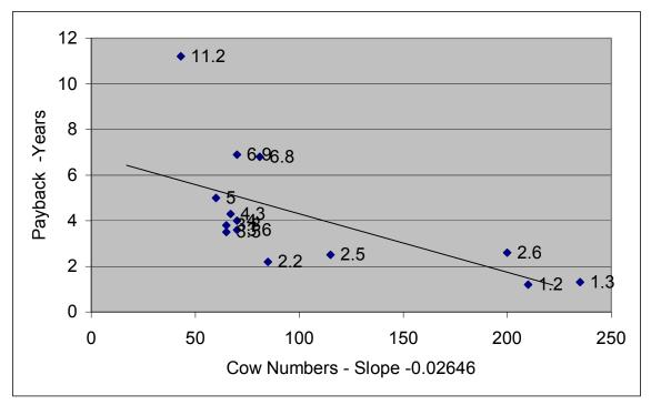
Figure 11: Plate Cooler Payback vs. Cow Numbers
