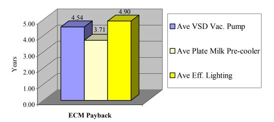
Figure 9: Simple Payback for Proposed ECMs – Tiestall and Freestall Farms
